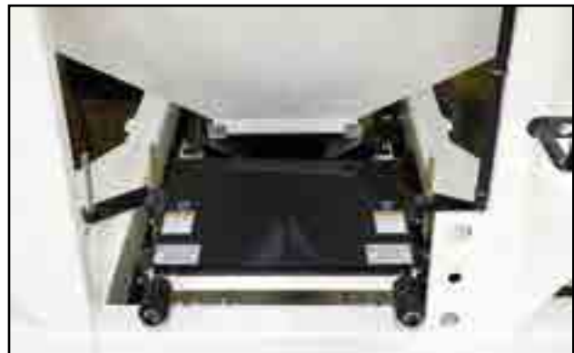
Fig 61 - Tension bolt on slave conveyor
