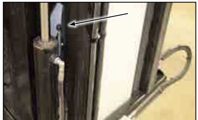
Fig 60 - Tension bolts on rear conveyor
