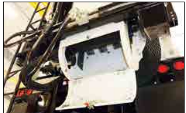
Fig 64 - Access door to paddle belt on rear conveyor
