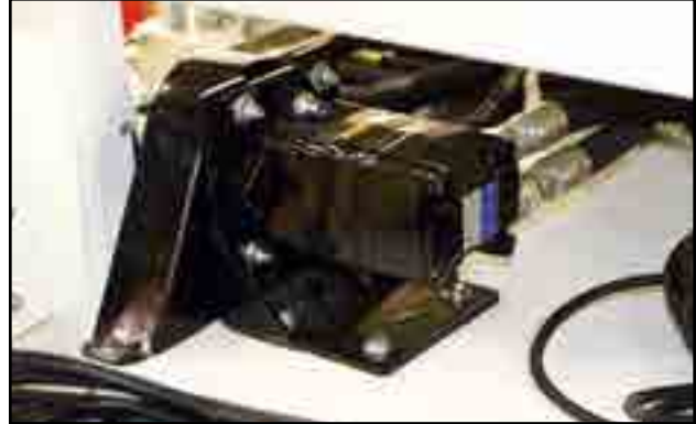
Fig 50 - Drive of slave conveyor
