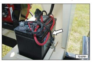
2. The battery is not charged when the engine is operating. If the battery is not charging using an external charger, check the fuse. Replace the fuse if necessary.
