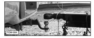
5. Lower the hitch onto the ball.
