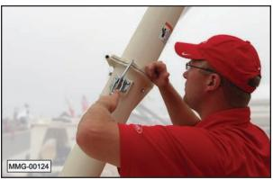
Note: Both auger tube sections use a spring loaded drive coupling. Even if the couplings are misaligned they will engage with each other once the auger begins to rotate.
