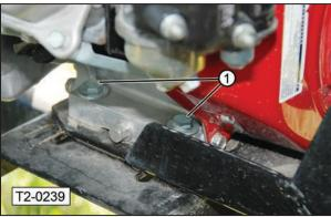
2. Loosen the engine base stabilizing bolt.
