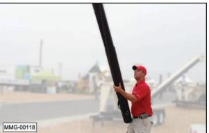
6. Lock the conveyor tube in place with the overcenter clamp.
