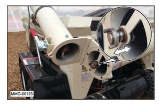
7. When not in use, place the end of the spout onto the bracket, as shown.
