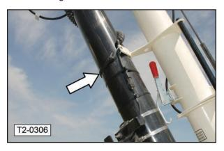
8. Place the delivery spout onto the storage bracket.
