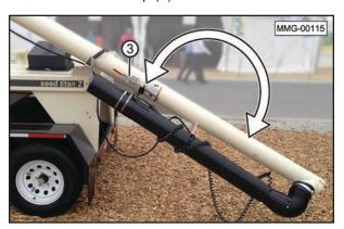
3. Release the retainer strap on the middle section of the conveyer tube.
