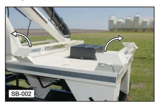
Remove the two hairpin retainer clips and remove the protective cover. Place the clips back into the retainer studs. Store the cover in a location that prevents it from being damaged.
