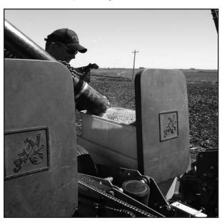
16. When the transfer of seed is complete, press the auger speed control switch to reduce the engine RPM and stop the auger.
