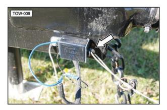
11. Route all the cables in a manner that will prevent snagging. Be sure to provide slack for turning.
