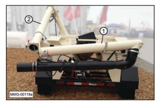
1. Release the retainer strap on upper tube (1) of the auger tube.
