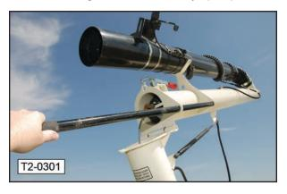
Unhook the auger tube retaining strap. Hold the end of the auger tube when releasing the retaining strap to prevent the tube from extending.
