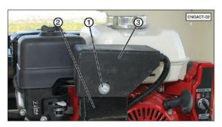
Ensure all personnel are clear of unit. Start the engine and test the actuator by pressing actuator switch (12) to ensure the engine speed increases and decreases as designed.
