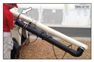
4. Remove the rubber retainer strap from the three-tier spout.
