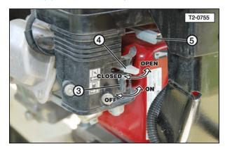
c. Turn the key switch to the ON position.
