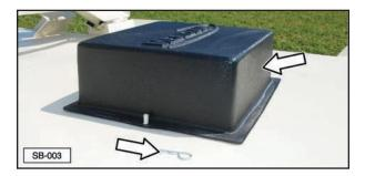
Make sure there are no foreign objects or impacted seed blocking the chute leading to the auger/conveyor.
