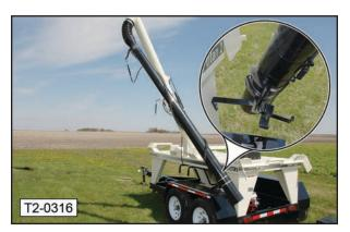
9. Lock the auger tube sections together using the over-center clamp.
