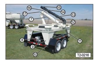
(8) Gas Cylinder (to assist raising auger).
