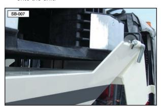
8. Make sure the rubber boot contacts the bottom of the seed box.
