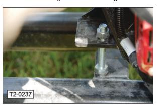
3. Loosen the jam nut on engine base adjusting bolt (2) and move the engine base to set the desired belt tension.
