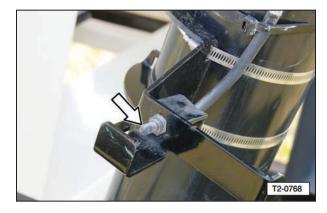
17. Close the slide gate by pulling the handle outward.
