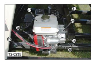
(25) Centrifugal Clutch Gearbox Oil Level.(26) Centrifugal Clutch (speed reduction for belt drive).(27) Fuel Tank.(28) Pull Start Rope.(29) Remote Throttle Switch Auxiliary Plug.
