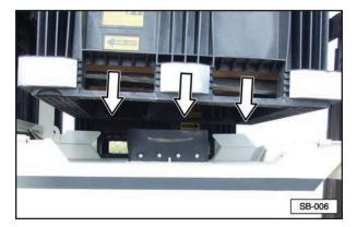
7. Make sure the seed box is loaded properly onto the unit.
