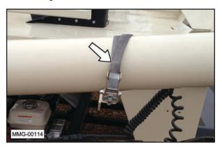
2. Open the upper tube and lock it in place with over-center clamp (3).
