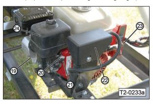
(19) Centrifugal Clutch Reduction Case.
