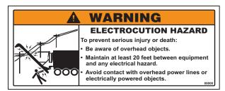
Check the surrounding area for structures or overhead power lines that would contact the conveyor in its raised position. Contact with electricity can result in serious personal injury or death.
