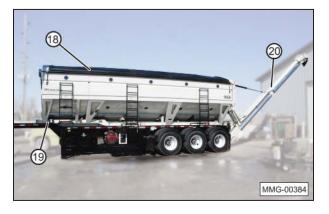
(18) Roll-up Tarp. (19) Bin Slide Gates and Cylinders. (20) Incline Conveyor in Unloading Position.
