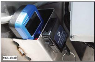
Wireless Remote Control Transmitter and Belt Tether Storage Location.
