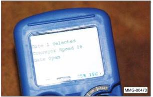
11. Set the desired conveyor speed by pressing the 'CONV ON' button additional times. Each press increases the speed by 25%.
