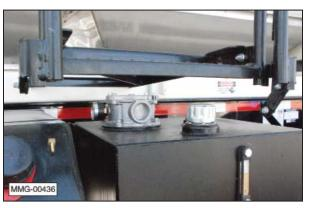
Annually, a sample of hydraulic oil should be taken to a dealer with oil analysis capability. When analysis shows the need to change the oil, use the following procedure. Use an AW HVI Hydraulic ISO 32 oil.
