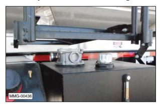
A hydraulic oil filter change is recommended annually or every 400 hours of operation, or whenever the oil filter flow gauge indicates the need for a filter change.
