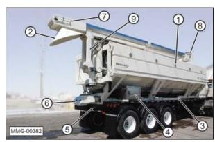
(1) Seed Compartments. (2) Hopper. (3) Seed Tender Frame. (4) Control Panel and Wireless Remote Control (not shown). (5) Trailer. (6) Underbin Conveyor. (7) Incline Conveyor in Transport Position. (8) Delivery Spout. (9) Pivot Frame.
