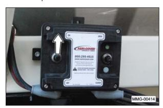
Open the tarp by pressing and holding the toggle switch. The tarp will stop when fully open, or may be stopped in any intermediate position by releasing the switch.
