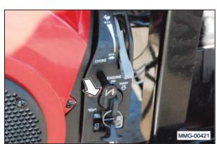
3. Move the throttle lever about 1/3 of the way to the MAX position.
