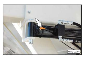
Cylinder Position Sensor Wires On Conveyor Slide/ Swing/Fold Cylinders.
