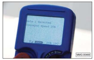
10. Open the slide gate for the desired compartment. Hold the button down until the gate is open to the desired amount. The gate will move while the button is depressed and will stop when the button is released or when fully open.
