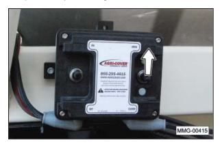
3. The tarp may be opened from the wireless remote by pressing SELECT, then pressing and holding the OPEN button.
