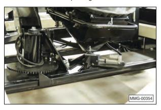
24. Press and hold the toggle switch upward to lock the ball coupling into the conveyor hitch receiver.
