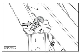
Once the tubes are locked together, move the toggle switch downward to unlock the conveyor hitch receiver (ball coupling) on the conveyor.
