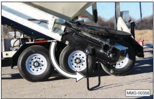
17. Raise the hopper by pulling the lock collar outward and lowering the handle. Lock the handle into place when the hopper is at the desired height.
