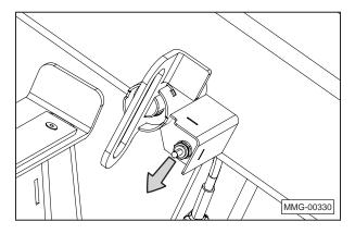
12. Rotate hopper guide handle 90° into the position shown.
