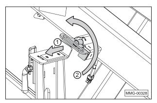
Release and push the lock pin inward to lock the inner and outer tubes of the conveyor arm together. Make sure the pin is fully engaged.
