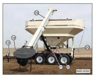
(18) Hopper and Cover. (19) Breakaway Trailer Brake System. (20) Transport Lock (Field and Road). (21) Pivot Platform. (22) Bin Slide Gates and Cylinders. (23) Conveyor in Self-loading Position.
