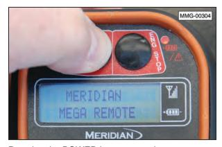
Pressing the POWER button turns the remote transmitter ON and displays the message "Meridian Mega Remote".
