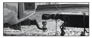
4. Lower the hitch onto the ball.
