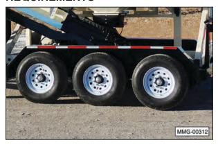
Initially check the wheel bolt torque at 5, 10, 25, and 50 miles and after each wheel removal.
