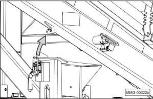
Using the remote control unit or the control panel, rotate conveyor to align the triangular indicator on the conveyor pivot plate with the alignment plate on the frame, as shown.
