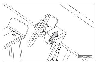
25. Pull out on locking pin and rotate 90° clockwise to shield toggle switch. Release the locking pin and make sure it is firmly seated in the open position.
