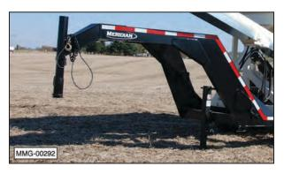
Adjust the trailer jack to set the trailer in a level position.
