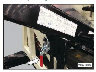
If not already removed, remove the protective cover from the seed pan. It may be necessary to lower the hopper in order to remove the cover. To lower the hopper, pull out on the sliding lock collar and raise the handle to lower the hopper.
