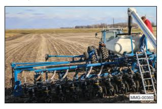
Position the hopper to prevent spillage of the seed. Make sure the handle is locked into the desired position before opening the seed compartment slide gates.
