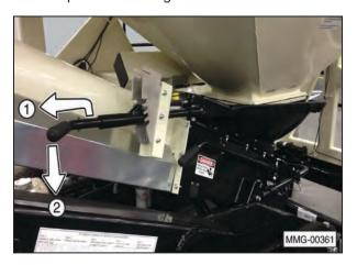
11. Manually start the conveyor or use the Auto Reset feature to automatically dispense a preselected amount of seed. Refer to section 5.4 Auto Reset Function for instructions.
