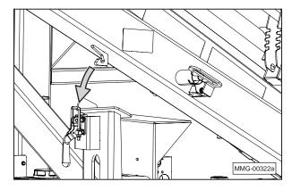
**NOTE:** Do not move the seed tender unless the conveyor is locked in the transport position.
