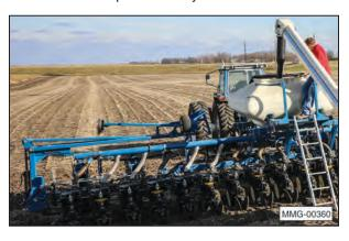
14. Return the conveyor to the transport position and latch before moving the seed tender.
