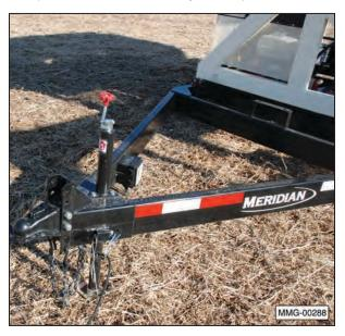
3. Slowly back the tow vehicle until the hitch and ball are aligned.
