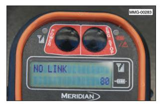
If the "NO LINK" message appears, the remote transmitter is not communicating with the control panel on the seed tender. Make sure the ON/OFF key switch is in the ON position.
