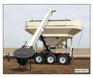
20. When the seed tender or other container is filled, stop the conveyor.
