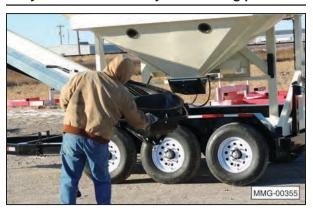
15. Use the conveyor left or the conveyor right buttons (switches) to position conveyor arm into the desired position. The photos show the self-filling position.
