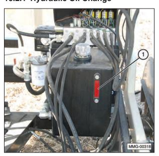
An oil and filter change is recommended annually or every 400 hours of operation using an AW HVI Hydraulic ISO 32 oil.
