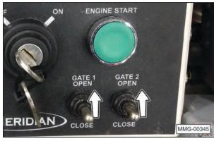
13. When the planter is filled, close the slide gate and then stop the conveyor belt.
