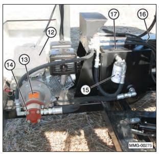
(12) Gasoline Engine to Power Hydraulic Pump.(13) Coupling (Engine to Pump). (14) Hydraulic Pump. (15) Hydraulic Oil Filter. (16) Hydraulic Tank Oil Level Sight Gauge. (17) Hydraulic Tank.
