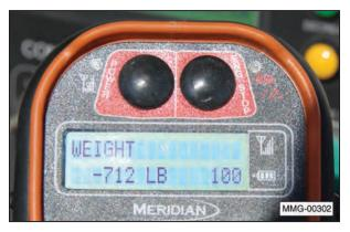
The remote transmitter will display the WEIGHT of the seed in the seed compartments in pounds. It also displays the battery life of the two AA batteries in a percentage of remaining life.
