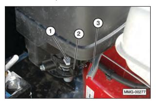
6. Start the engine and move throttle lever (3) to run the engine at full speed.
