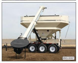
If desired, release the stand lock pin and rotate the stand downward. Engage the lock pin when the stand is fully extended.
