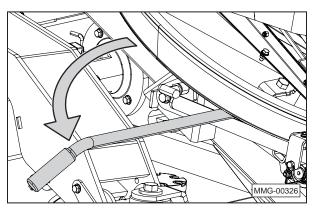
13. Slide the ball coupling out of the conveyor hitch receiver.
