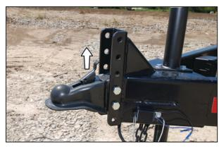
5. Slowly back the tow vehicle until the hitch and ball are aligned.
