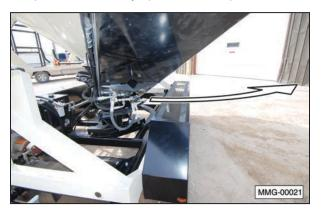
9. Raise or lower the conveyor tube to the desired height.
