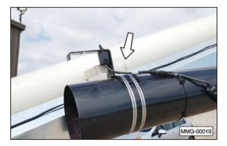
6. Remove the delivery spout from the retaining bracket and rest it on the ground.
