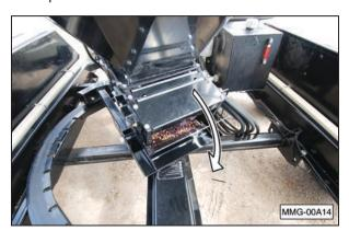
2. Position the crimped belt fastener in the opening.
