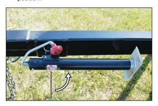
8. Close the receiver locking collar using the lever. Install the retainer clip to prevent unwanted opening of the receiver.
