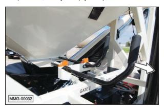
12. Hold the delivery spout handle and manually start the conveyor by moving the switch to the ON position.
