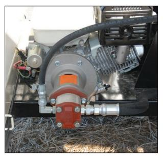
Remove the orange protective cover from the adapter assembly.
