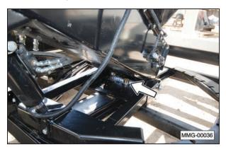
4. Make sure the tarp roll up cable is tensioned correctly. Refer to the OEM manual for additional information.
