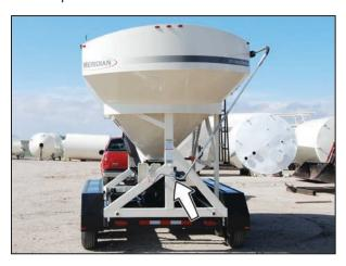
5. Two cables (1) are used to provide proper tarp tension. Use ratchet tighteners (2) to adjust the cable tension.
