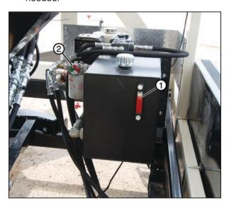
Check the filter life indicator. Change the filter if the indicator needle is in the yellow or red area.
