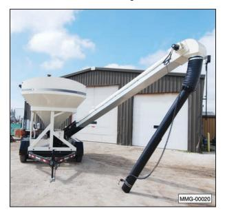
7. Using the conveyor tube raise/lower lever, slightly raise the conveyor out of the storage cradle.
