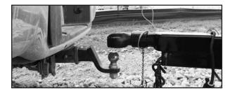
6. Lower the hitch onto the ball.
