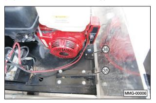
(35) Frame-to-Trailer Hold-down Brackets. (36) Rectifier (charges battery when engine is running).
