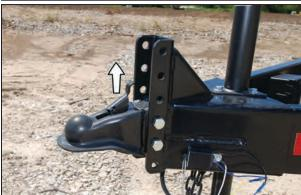
5. Slowly back the tow vehicle until the hitch and ball are aligned.
