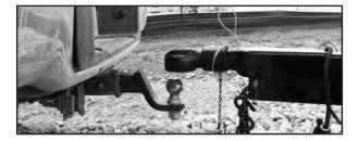
6. Lower the hitch onto the ball.
