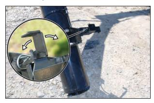
12. Open the seed compartment slide gate by pushing the handle inward. Close the slide gate by pulling the handle outward.
