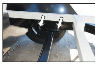
The front hitch section of the seed tender is bolted to the trailer frame. This design allows the same trailer to use either a standard bumper hitch assembly or a gooseneck trailer hitch if this option is available.
