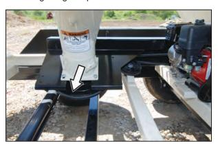
Use a screwdriver to reset the high idle stop screw if required to obtain the desired speed.
