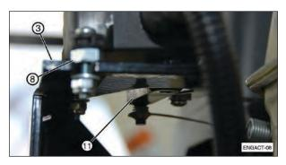
b. If actuator arm (11) is below the bracket (as shown), the arm will continue to rotate and not function properly. The bracket serves as a stop for the arm.
