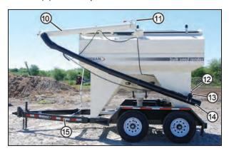
(10) Auger Tube. (11) Auger Tube Clamp.(12) Delivery Spout Holder. (13) Auger/Engine Throttle Switch. (14) Delivery Spout. (15) Bolt-On Bumper Hitch Tongue Assembly.
