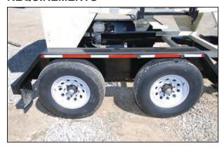
Initially check the wheel bolt torque at 10, 25, and 50 miles and after each wheel removal. Refer to the Wheel Bolt Torque Requirements section in this manual for tightening instructions.
