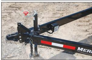
3. Adjust the receiver height to make the trailer level with the tow vehicle. Tighten the bolts to 70 ft-lb (95 N⋅m) torque.
