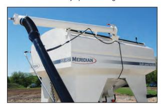
Make sure the auger cable is threaded into the hole in the end of the auger. Damage to the auger can occur if the cable is not properly inserted.
