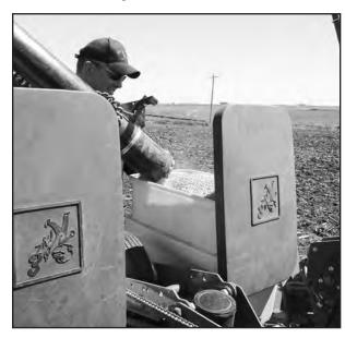
14. When the transfer of seed is complete, press the auger speed control switch to reduce the engine RPM and stop the auger.
