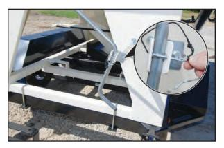
Extend the crank handle assembly to a comfortable operating position.
