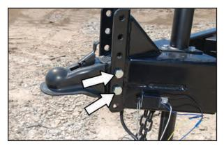
4. Remove the retainer pin. Release or open the receiver by pulling the locking cover back using the lever mechanism, as shown.
