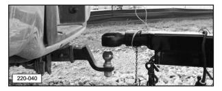
5. Lower the hitch onto the ball.
