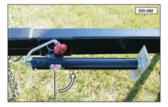
7. Close the receiver locking collar using the lever. Install the retainer clip to prevent unwanted opening of the receiver.
