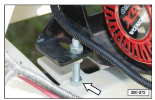
3. Loosen engine base adjusting bolt jam nut and move engine base to set the desired belt tension.
