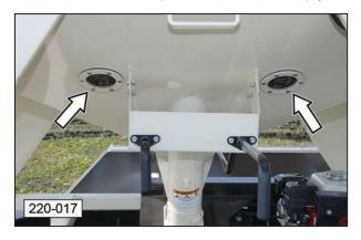
4. When the compartment is filled, close the cover(s) and lock it in place with the rubber latch.
