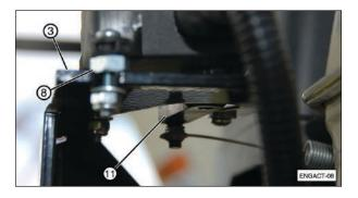
b. If actuator arm (11) is below the bracket (as shown), the arm will continue to rotate and not function properly. The bracket serves as a stop for the arm.
