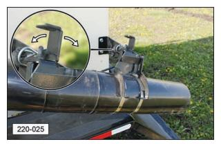
13. Open the seed compartment slide gate by pushing the handle inward. Close the slide gate by pulling the handle outward.
