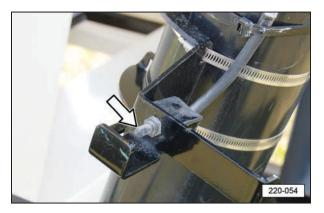
16. Close the seed compartment slide gate by pulling the handle outward.
