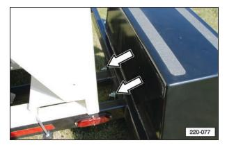
The front hitch section of the seed tender is bolted to the trailer frame. This design allows the same trailer to use either a standard hitch assembly or a gooseneck trailer hitch if this option is available.
