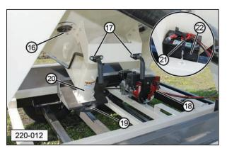
(16) Compartment View Glass. (17) Slide Gate Levers. (18) Gasoline Engine. (19) Auger Drive Pulley. (20) Auger Tube Clean Out Door.
