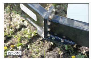
Check the torque on the frame hold-down bolts at least once per year. Tighten the bolts to 40 ft-lbs.
