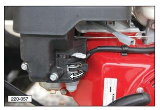
19. Before towing the unit on the road, return the auger tube and delivery spout to its stored position. Latch the rubber tie-down strap over the delivery spout.
