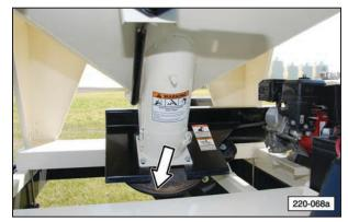
3. Use a screwdriver to reset the high idle stop screw if required to obtain the desired speed.
