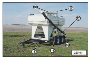
(10) Auger Tube. (11) Auger Tube Clamp.
