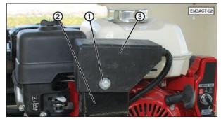
Ensure all personnel are clear of unit. Start the engine and test the actuator by pressing actuator switch (12) to ensure the engine speed increases and decreases as designed.
