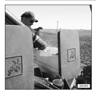
15. When the transfer of seed is complete, press the auger speed control switch to reduce the engine RPM and stop the auger.
