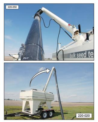
8. Lock the auger tube to the seed tender using the over-center clamp.
