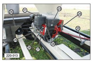
(23) Auger-Speed Actuator. (24) Gas Engine On/Off Controls. (25) Remote Throttle Switch Auxiliary Plug. (26) Throttle Lever (connected to auger speed actuator). (27) Choke Lever.
