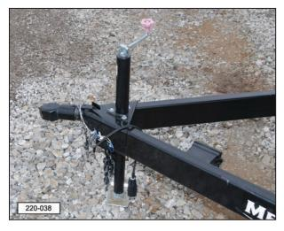
3. Remove the retainer pin. Release or open the receiver by pulling the locking cover back using the lever mechanism, as shown.
