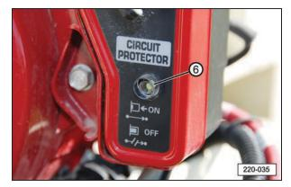
6. Engine Circuit Protection The circuit protector protects the battery charging circuit. A short circuit, or a battery connected with reverse polarity, will trip the circuit breaker. The green indicator inside the circuit protector will pop out to show that the circuit protector has switched off.
