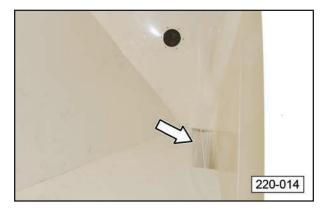
**NOTE:** Two view windows, one in each compartment, can be used to determine the type of seed in the compartment and when the compartment is almost empty.
