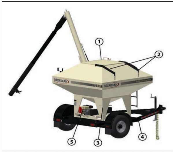
(1) Seed Bin Cover. (2) Seed Bin Cover Rails. (3) Seed Tender Frame. (4) Trailer. (5) Gasoline Engine.
