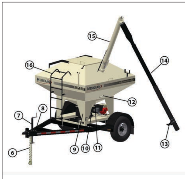
(6) Trailer Safety Chains. (7) Jack Stand. (8) Break-Away Trailer Brake System. (9) Document Storage Tube (inside of frame). (10) Delivery Spout Storage Bracket. (11) Slide Gate Lever. (12) View Glass. (13) Auger/Engine Throttle Switch. (14) Delivery Spout. (15) Auger Tube. (16) Ladder.
