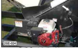
Fig 47 - Remote throttle switch
