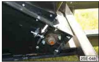
Fig 71 - Conveyor belt tension bolt
