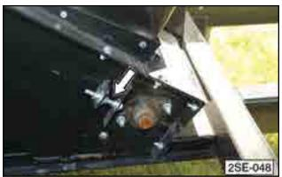
Fig 74 - Belt Tension bolts
