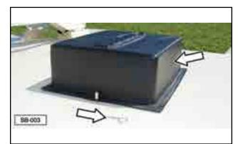
Fig 34 - Remove protective chute cover
