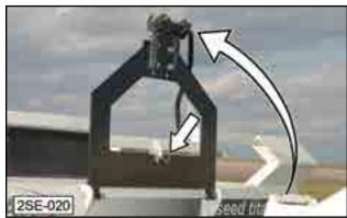
Fig 40 - Raise Titan 2SE lock plate
