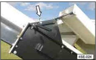
Fig 14 - Conveyor tube transport lock
