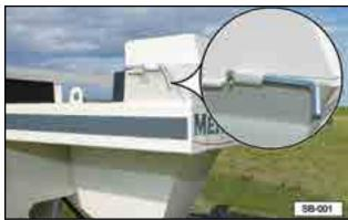
Fig 32 - Lock-down arm and latch pin
