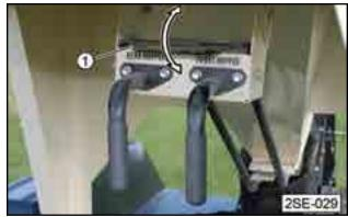
Fig 51 - Lift lock plate to use slide gate handles
