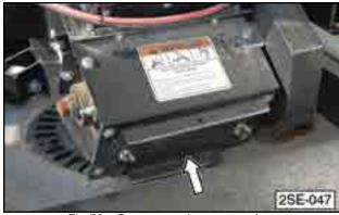
Fig 73 - Conveyor tube access door
