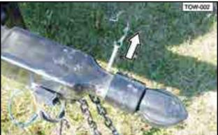
Fig 25 - Hitch receiver Retainer pin
