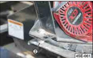
Fig 67 - Titan 4SE engine base stabilizing bolts
