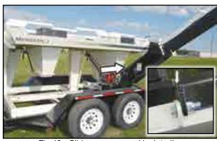
Fig 43 - Slide conveyor and lock trolley
