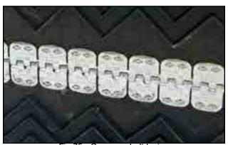
Fig 75 - Conveyor belt lacing
