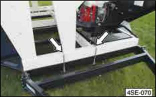
Fig 84 - Titan 4SE frame hold-down bolts
