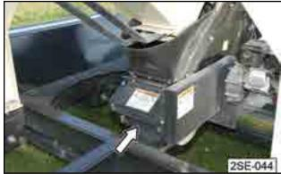
Fig 77 - Conveyor tube access door
