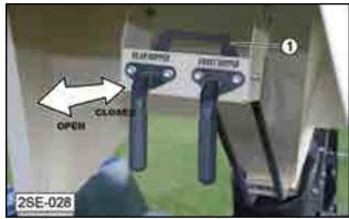
Fig 52 - Lock plate in "locked/closed" position
