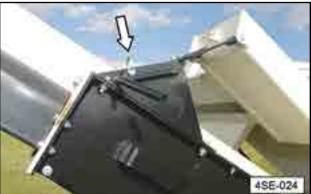
Fig 41 - Lock plate handle on Titan 4SE
