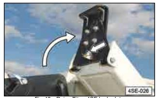
Fig 42 - Raise Titan 4SE lock plate
