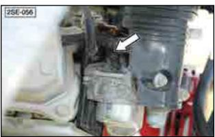
Fig 60 - Engine speed setscrew
