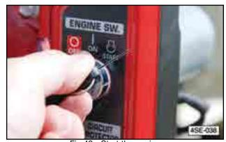
Fig 49 - Start the engine
