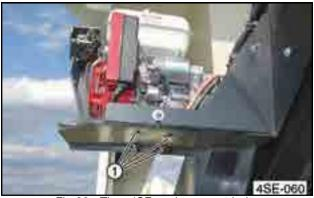
Fig 66 - Titan 4SE engine mount bolts
