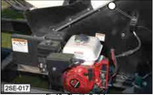
Fig 12 - Throttle Switch
