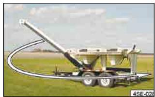
Fig 46 - 4SE tube shuttle and swing
