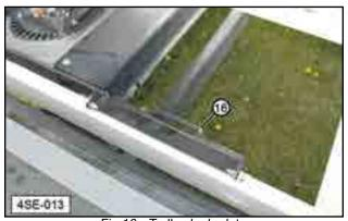
Fig 16 - Trolley lock plate
