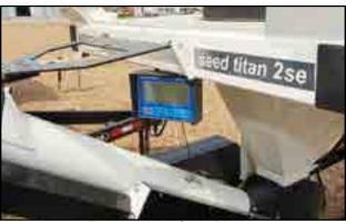
Fig 22 - Weigh Scale Display
