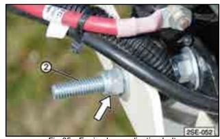
Fig 65 - Engine base adjusting bolt
