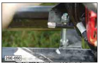
Fig 64 - 2SE Engine base stabilizing bolts
