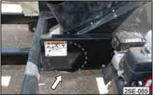
Fig 61 - Drive belt pulley inside guard
