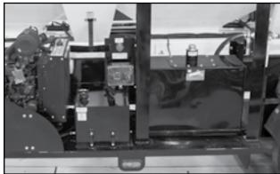
Fig 45 - Fuel tank and hydraulic oil reservoir
