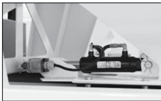
Fig 37 - Compartment gate cylinder
