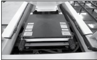
Fig 58 - Slave conveyor tension bolt and springs
