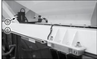
Fig 18 - (a) Load Cell, (b) weigh scale junction box
