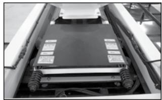
Fig 56 - Slave conveyor tension bolt and springs
