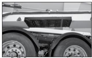
Fig 62 - Rear conveyor, access panel removed
