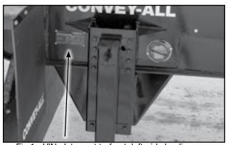
Fig 1 - VIN plate next to front, left-side landing gear
