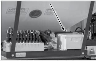
Fig 16 - Remote control receiver box
