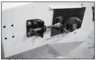
Fig 51 - Adjustment bolt, rear conveyor discharge
