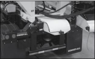
Fig 13 - Slave discharge spout
