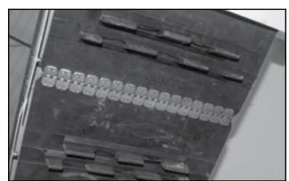
Fig 63 - Alligator lacing on rear conveyor paddle belt
