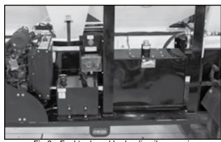
Fig 9 - Fuel tank and hydraulic oil reservoir
