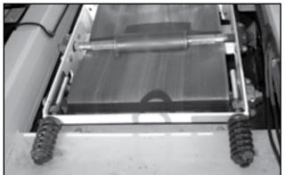
Fig 50 - Slave conveyor tension bolts, cover removed
