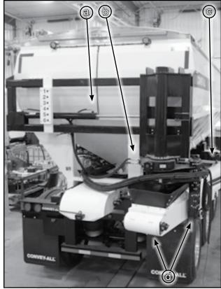
Fig 48 - Rear conveyor movement points
