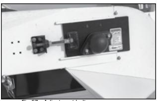
Fig 57 - Adjustment bolts on rear conveyor
