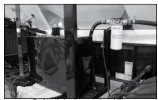
Fig 64 - Hydraulic reservoir and filter
