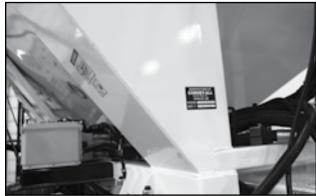
Fig 2 - Serial # on rear, left-side, vertical beam
