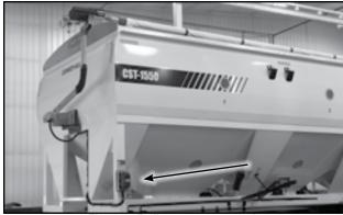
Fig 21 - Roll-top tarp controls
