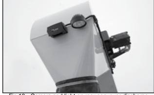
Fig 19 - Camera and light on rear conveyor discharge
