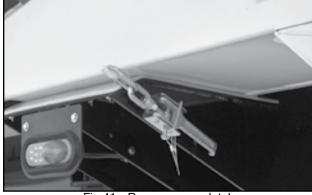
Fig 41 - Rear conveyor latch
