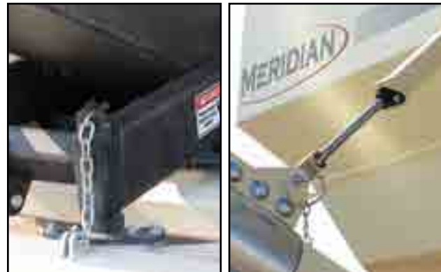
Fig 47 - Secure conveyor tube for transport
