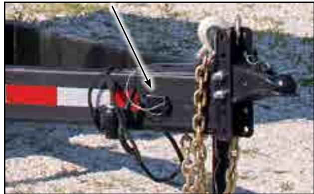
Fig 17 - Break-Away cable on hitch tongue
