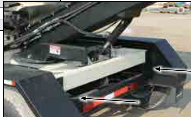
Fig 67 - Weigh scale load cell location
