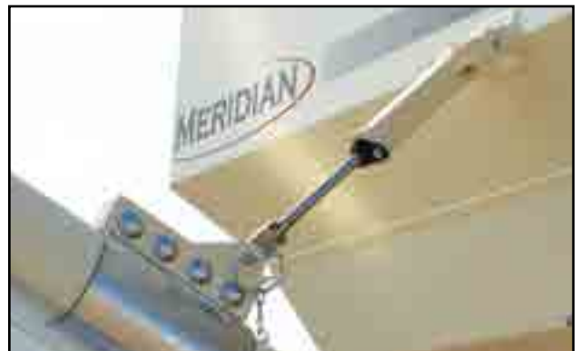
Fig 43 - Conveyor tube transport lock and damper mechanism
