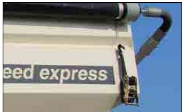
Fig 36 - Tarp tension ratchet straps
