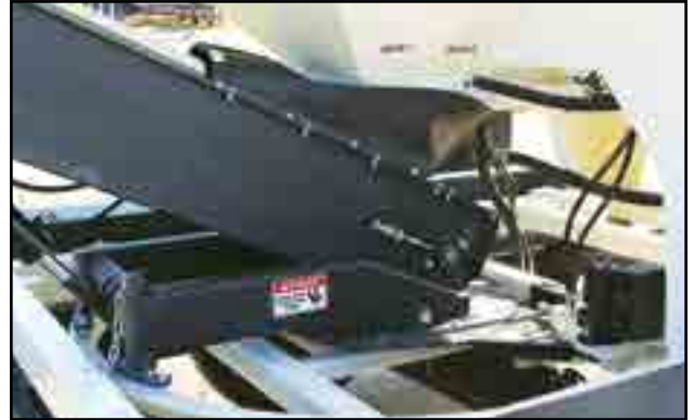
Fig 41 - Conveyor hopper on turntable platform
