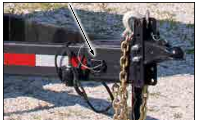
Fig 64 - Break-Away cable on hitch tongue
