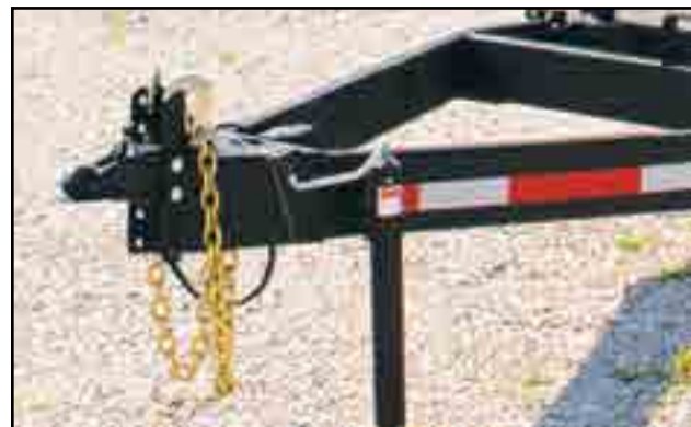
Fig 27 - Trailer hitch with safety chains
