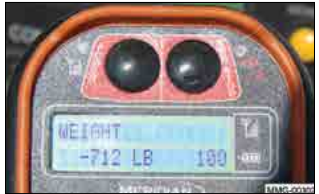
Fig 23 - Handset displays weight
