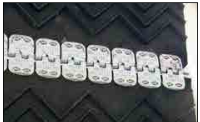
Fig 59 - Conveyor belt lacing
