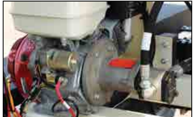
Fig 54 - Engine and hydraulic pump
