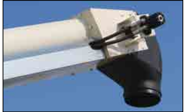
Fig 12 - Conveyor discharge spout
