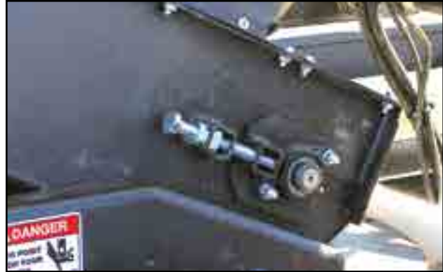
Fig 56 - Hopper roller tension bolt
