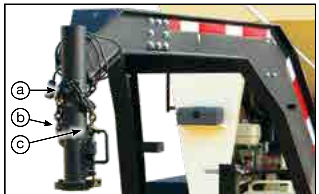
Fig 31 - Gooseneck hitch components
