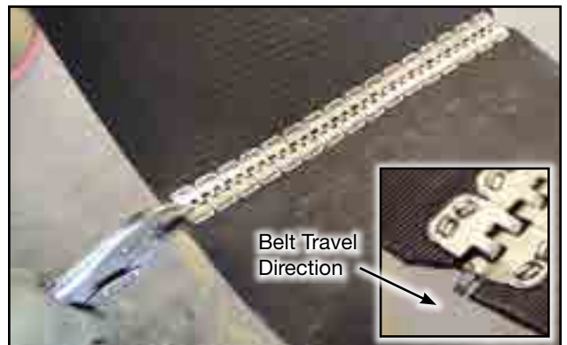
Fig 60 - Crimp lacing and taper belt corner
