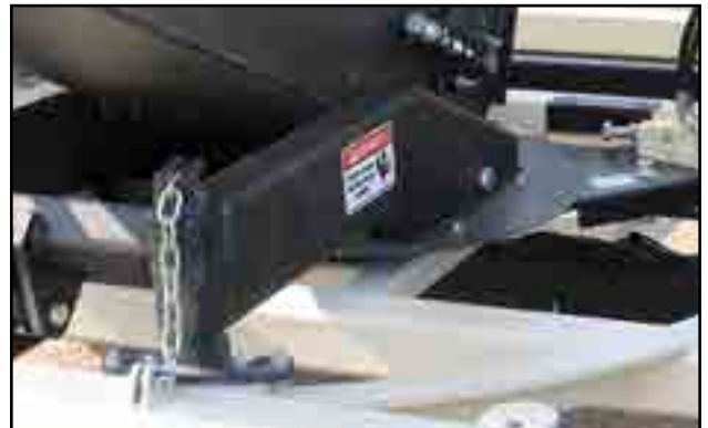
Fig 42 - Turntable platform anti-rotation chain
