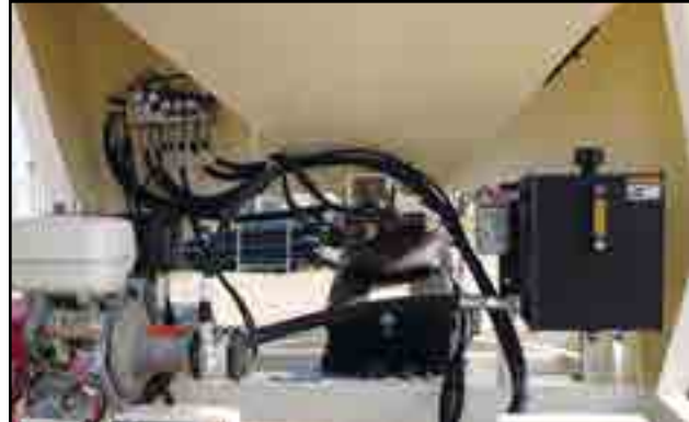
Fig 8 - Engine, hydraulic oil reservoir and filter
