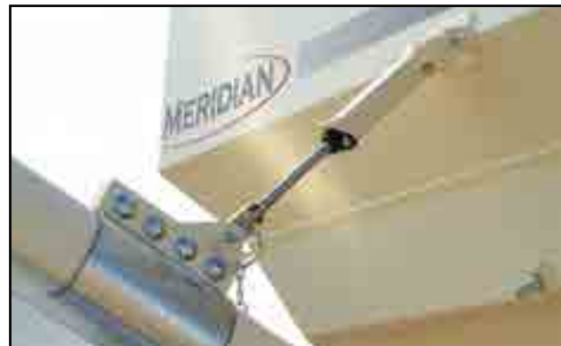
Fig 26 - Conveyor tube transport lock w/ damper mechanism
