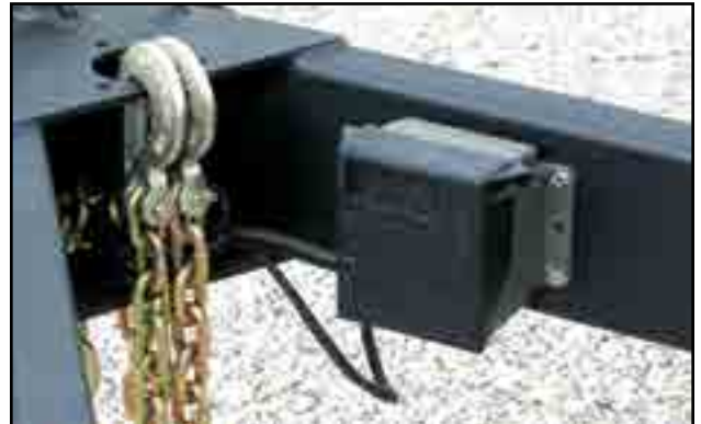
Fig 63 - Break-Away system control box
