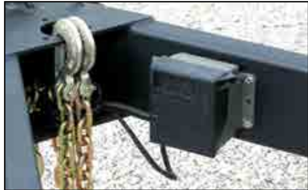
Fig 16 - Break-Away system control box
