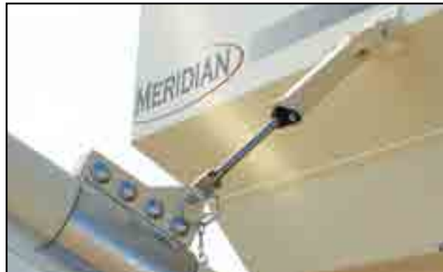
Fig 10 - Conveyor tube damper mechanism and transport lock
