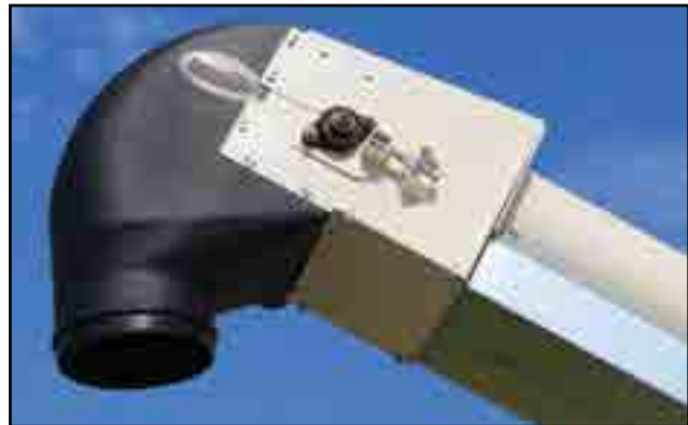
Fig 57 - Discharge adjustment bolt
