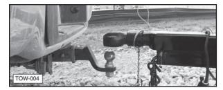
5. Lower the hitch onto the ball.
