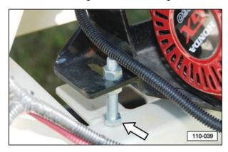
3. Loosen the engine base adjusting bolt jam nut and move the engine base to set the desired belt tension.
