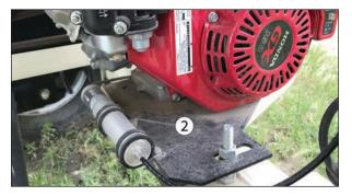
3. Loosen screw on wire holder, (3).and loosen screw on cable holder (4).Then remove the actuator cable from the holders.
