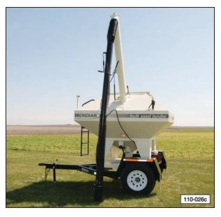
8. Lock the auger tube to the seed tender using the over-center clamp.
