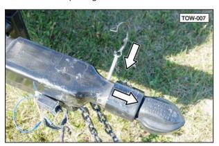
8. Attach the safety chain securely to the tow vehicle to prevent unexpected separation. Cross the chains when attaching.
