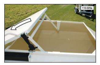
4. When the bin is filled, close the cover and lock it in place with the rubber latch.
