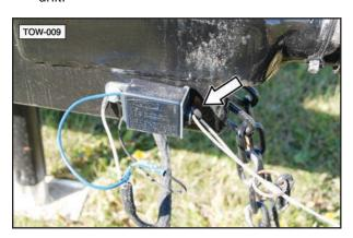
Route all the cables in a manner that will prevent snagging. Be sure to provide slack for turning.
