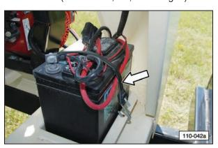
The battery is not charged when the engine is operating. If the battery is not charging using an external charger, check the fuse. Replace the fuse if necessary.
