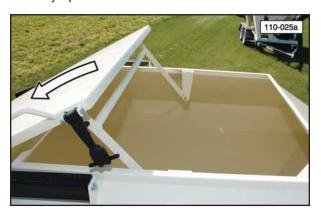
5. When the bin is filled, close the cover and lock it in place with the rubber latch.
