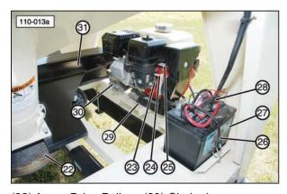
(22) Auger Drive Pulley. (23) Choke Lever.
