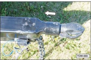
4. Slowly back the tow vehicle until the hitch and ball are aligned.
