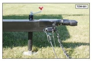
Remove the retainer pin. Release or open the receiver by pulling the locking cover back, as shown.
