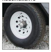
Initially check the wheel bolt torque at 10, 25, and 50 miles and after each wheel removal. Refer to the Wheel Bolt Torque Requirements section in this manual for tightening instructions.
