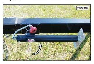
7. Close the receiver by pulling the spring loaded locking collar back to release the hitch mechanism. Install the retainer clip to prevent unwanted opening of the receiver.
