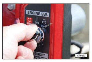
12. If necessary, decrease the engine speed below 1400 RPM using the remote throttle control switch. A centrifugal clutch on the engine will engage and rotate the auger when the engine speed exceeds 1400 RPM. Increasing the engine speed will increase the unloading rate.
