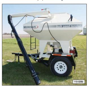
Make sure the auger cable is threaded into the hole in the end of the auger. Damage to the auger can occur if the cable is not properly inserted.
