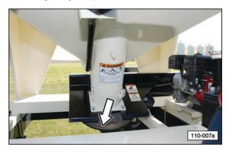
3. Use a screwdriver to reset the high idle stop screw if required to obtain the desired speed.
