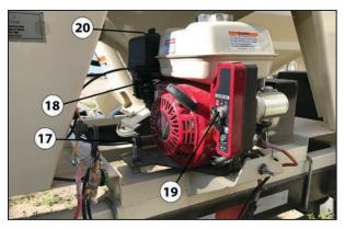
(17) Auger-Speed Actuator. (18) Gas Engine Controls. (19) Gas Engine On/Off Controls.(20) Air Filter.
