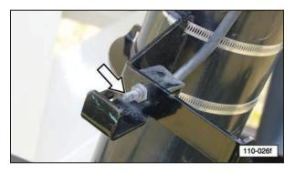
13. Open the seed slide gate by pushing the handle inward. Close the seed slide gate by pulling the handle outward.
