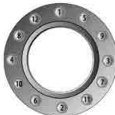
Fig 26 - 12 Bolt sequence
