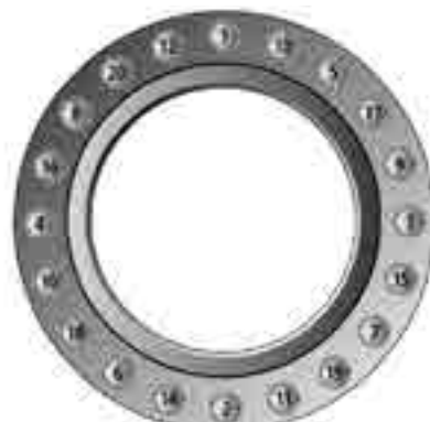
Fig 28 - 20 Bolt sequence
