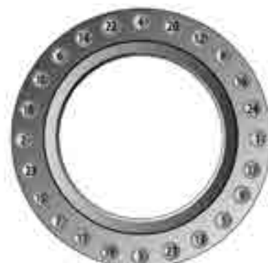
Fig 29 - 24 Bolt sequence
