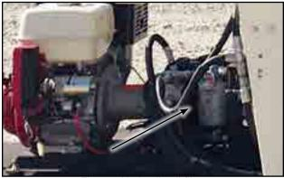
Fig 45 - Hydraulic oil filter
