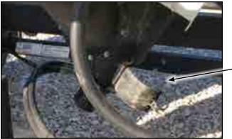
Fig 48 - Bottom clean-out access door
