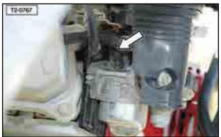
Fig 44 - Engine speed setscrew
