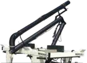
Fig 13 - Auger tube folded for transport and storage
