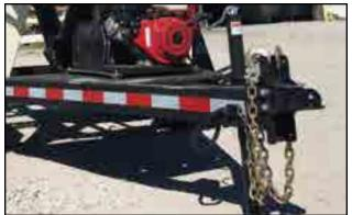
Fig 23 - Hitch receiver
