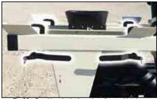
Fig 28 - Seed box lock-down handles and latches
