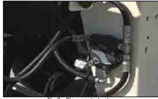
Fig 8 - Flow control valve
