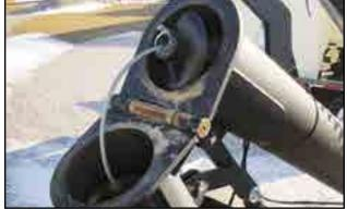
Fig 35 - Auger drive coupling
