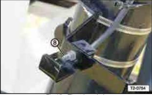
Fig 15 - Throttle switch
