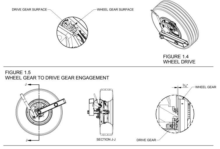
Once welding is complete, recheck gear engagement. If more engagement is required, the outer 1/2" flange nut can be loosened at the bottom of the handle. The 1" slot in the bottom of the handle will allow the handle to be lifted up which will mesh the drive gear deeper into the wheel gear.
