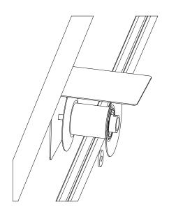
Once the pulley is in proper alignment the belt should track evenly in the center of the pulley.
