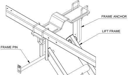
Install the Lift Arm between the Lift Frame and slide the Frame Pin all the way through.
