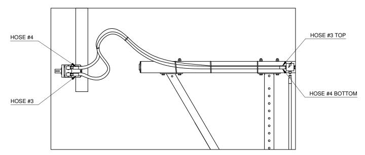
Install two drive motor fittings onto each of the drive motors. Then install the #3 and #4 hoses into the cushion block as shown above. Now run the hoses along the axle to the left and shape hoses into an "S" shape and hook up to the LH drive motor ports as designated.
