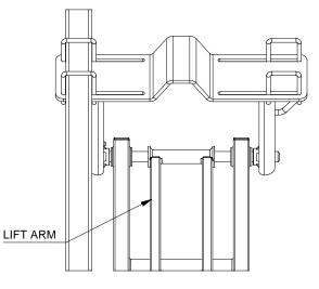
Secure Frame Pin with  $\frac{5}{16}$ " X 1" - NC bolt and  $\frac{5}{16}$ " spring washer.
