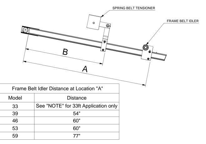
**Note:** On the 33 ft only, mount the idler on the bottom of the frame 5/8" from the cylinder base frame mount and flush with the top.
