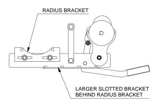
The big block pump has a small radius mounted stationery bracket that bolts on with two 7/16" x 1-1/2" bolts. It has a larger slotted bracket fastened to the back side of the stationary bracket which allows belt tensioning.
