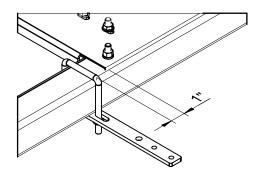
Secure filter mounting bracket with 2-1/2" or 3" U-bolt, depending on frame size, 1" ahead of the winch mounting plate.
