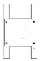
Use the set of holes which position the plate closest to the intake.
