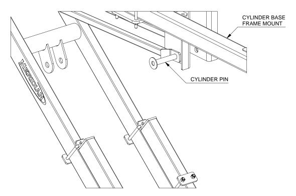
Install base end of the hydraulic cylinder into the Cylinder Base. Note the position of the hydraulic cylinder fitting ports. Push the 3/4" X 5" cylinder pin through the cylinder pin boss and the other side of the Cylinder Base. Install the 3/4" SAE washer and 3/16" X 1-1/2" cotter pin to retain the cylinder pin. Securely tighten all the U-bolts and lock nuts on the Cylinder Base.
