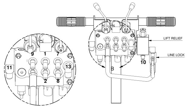
Connecting drive circuit hoses #1 & #2 from control valve to the cushion block
