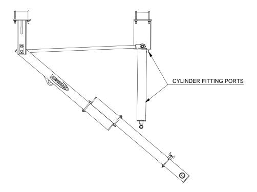
Swing the rod end of the hydraulic cylinder up and align with pin bosses on the Main Frame Cylinder mount. Install the 3/4" X 3-1/2" cylinder pin. Install the 3/4" SAE washer and 3/16" X 1-1/2" cotter pin to retain the cylinder pin.
