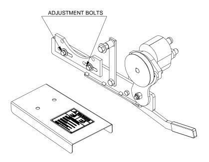
After installing the drive pulley, the belt (BX-34) can be installed. Provide slight tension to the two 3/8" adjustment bolts at the bottom of the radius bracket. Pull back on the pump bracket, tightening the adjustment bolts. This step may be repeated until proper belt tension is attained. Preferred tension is 20lbs per ¼" belt deflection. Install the belt guard.
