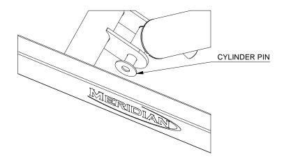
Support the Lift Frame assembly with a hydraulic jack or blocking to provide approximately 22" between the walking beam pin and the floor to aid installation of the walking beams.
