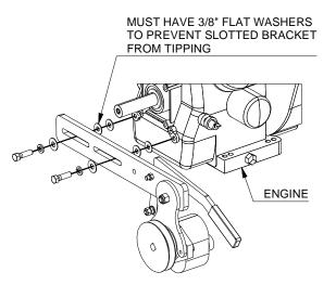
To mount the pump, first install a 7/16" lock washer and 7/16" flat washer onto the 7/16" x 1-1/2" bolt. Insert the bolt through the slotted bracket, then install two 3/8" flat washers onto the bolt and insert into the 7/16" engine block mounting holes. Note: there are four 3/8" completely round flat washers to be used on the Vanguard engines. There are four 3/8" flat washers that are nipped off on the edge to fit the Kohler engines.
