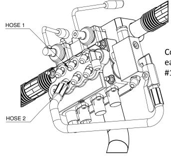
Connect #2 hose first and then #1 to ease installation as it is below fitting #1.
