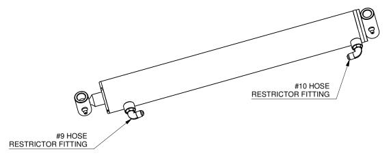
Connect #9 hose to the rod end of cylinder and the #10 hose to the base end of the cylinder.
