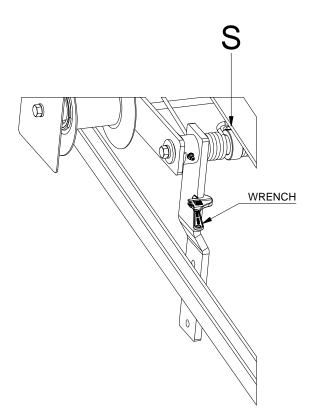
There is also an adjustment to be made on the spring if more spring tension is required. Spring adjustment is done by loosening the square headed set screw "S" on the shaft collar. With the belts out of the way from the pulley, lower the pulley down allowing the spring to move down and retighten the set screw. Lift pulley up and place belts back under the pulley and test for required tightness.
