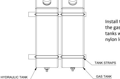
Install the hydraulic oil tank to the inside and the gas tank to the outside. Fasten down the tanks with the four tank straps and 5/16" nylon lock nuts.
