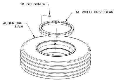
FIGURE 1.1 WHEEL GEAR INSTALLATION
