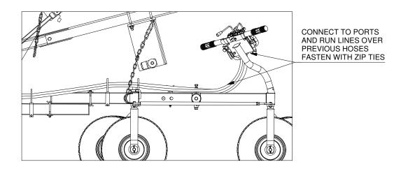
Connect the #8 hose to the "T" fitting on the winch motor and the #7 hose to the fitting on the silver relief valve block.
