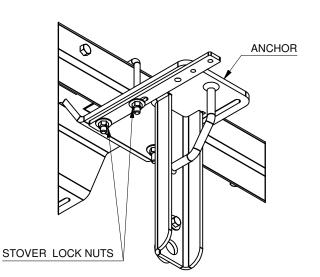
Secure filter mounting bracket to bottom of Anchor using the 3/8" Stover lock nuts.
