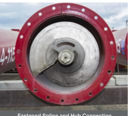
Fastened Spline and Hub Connection
