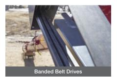
Our banded belt drive gives you better grip on drive pulleys and eliminates single belt slipping. Combine it with our electric clutch for smoother operation and less whipping.
