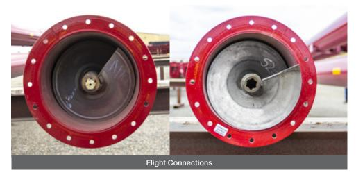
Meridian 10" and 12" swing augers, feature a spline and hub flight assembly connection. This unique connection, allows for movement without adding additional strain on the top head end and bottom boot bearings.
