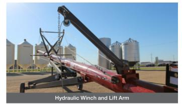
Raise or lower the hopper and swing tube with ease. The lift arm and winch can be quickly mounted on the left or right of the tube, allowing for unloading from either side of the swing auger.
