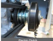
Designed specifically for the auger industry, our clutch can accommodate double-beltdrive and triple-belt-drive augers and can shut down the auger flighting, even from inside the bin.
