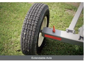
Meridian swing augers features a standard extendable axle. 10" & 12" SLMD axle shown above.
