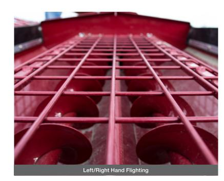
Meridian was the original designer and patent holder of left/right hand hopper flighting. Meridian's left and right hand flighting ensures fast and efficient flow into the main tube.
