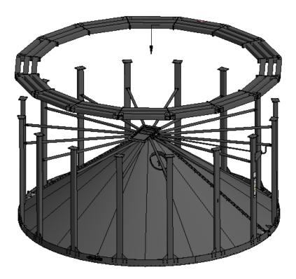
4. Once the skid is assembled, flip the completed hopper assembly into upright position. Install the crank and any other remaining items.
