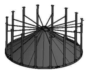
3. Assemble the skid on the ground. Install the assembled skid onto the assembled hopper with legs.
