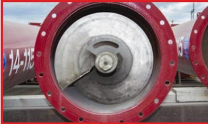
Fastened Spline and Hub Connection
