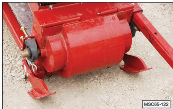
9. If removed, reinstall the discharge hood.
