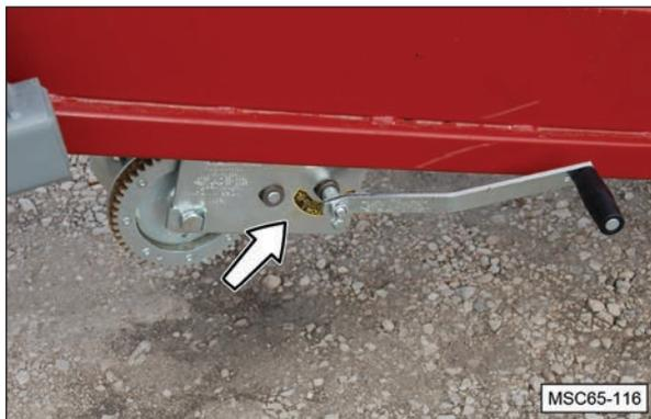
3. For manual winch operation, turn the crank clockwise to raise the conveyor and counterclockwise to lower it.
