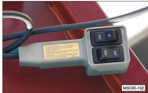
1. The remote control switch has two rocker switches to control the electric winch.
