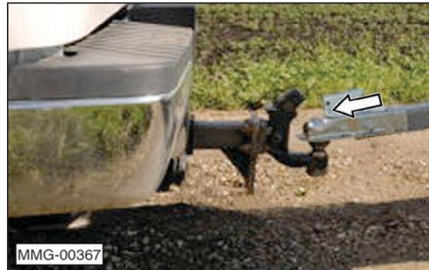
5. If equipped, place the jack in its stowed position.
