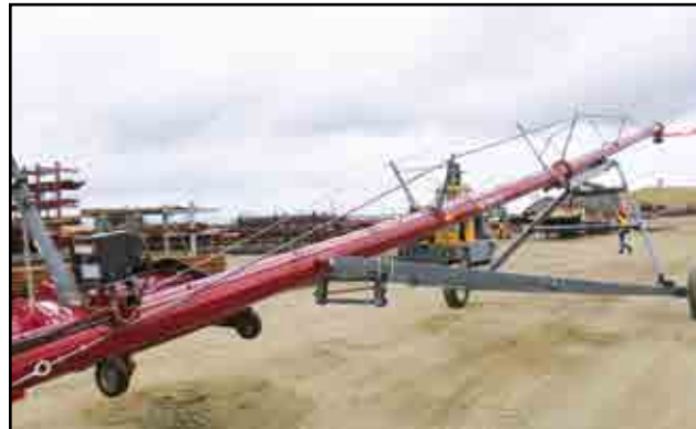
Fig 18 - Upward bow in auger tube
