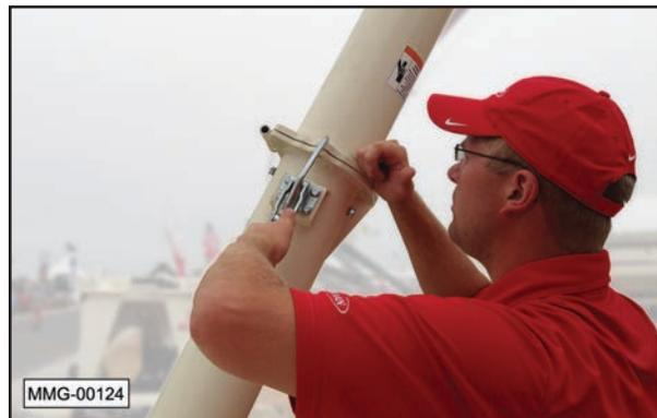
Note: Both auger tube sections use a spring loaded drive coupling. Even if the couplings are misaligned they will engage with each other once the auger begins to rotate.
