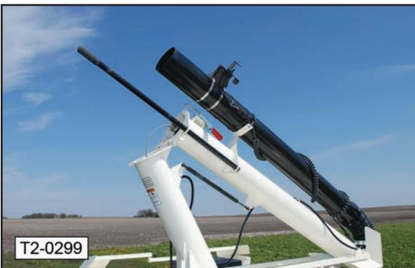
6. Pull the auger tube into the fully open position.
