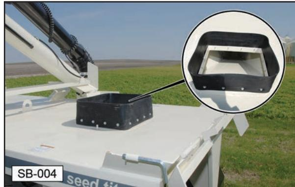
5. Make sure frame is clear of debris and stand clear when placing the seed box onto the seed tender.
