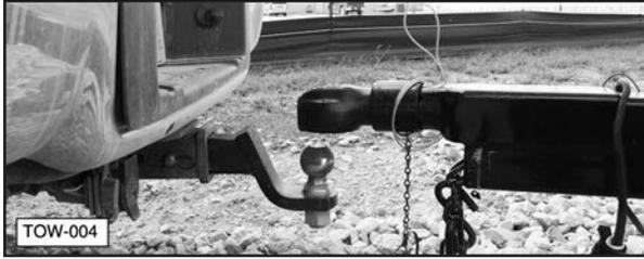
5. Lower the hitch onto the ball.
