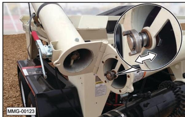
7. When not in use, place the end of the spout onto the bracket, as shown.
