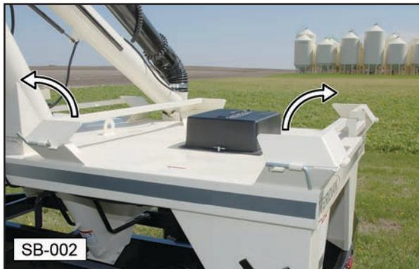
3. Remove the two hairpin retainer clips and remove the protective cover. Place the clips back into the retainer studs. Store the cover in a location that prevents it from being damaged.
