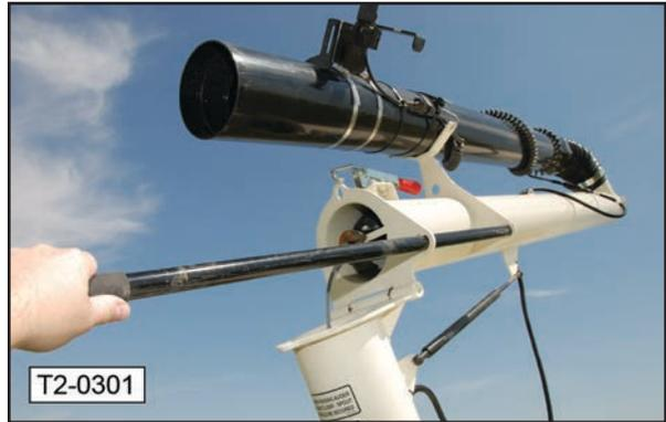
7. Unhook the auger tube retaining strap. Hold the end of the auger tube when releasing the retaining strap to prevent the tube from extending.
