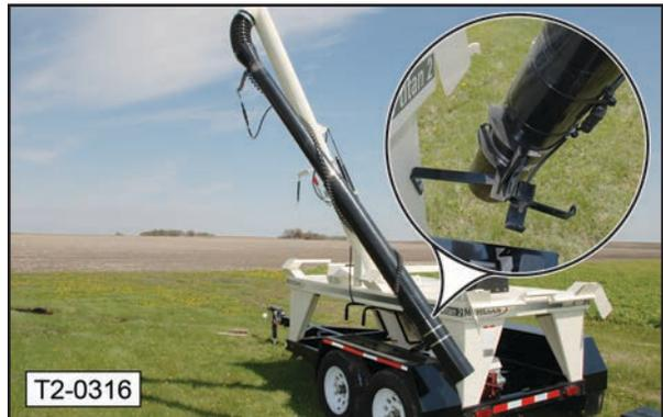
9. Lock the auger tube sections together using the over-center clamp.
