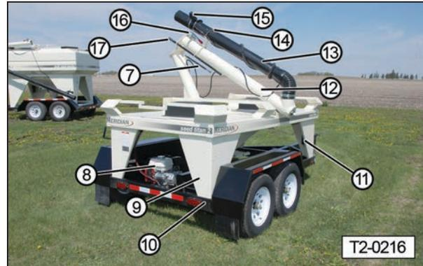
(8) Gas Cylinder (to assist raising auger). (9) Gasoline Engine. (10) Seed Box Frame. (11) Trailer Frame. (12) Document Storage Tube (inside frame). (13) Auger (upper section). (14) Discharge Spout. (15) Retainer Strap. (16) Engine Speed Control Switch. (17) Auger Latch. (18) Handle (for raising/lowering auger).
