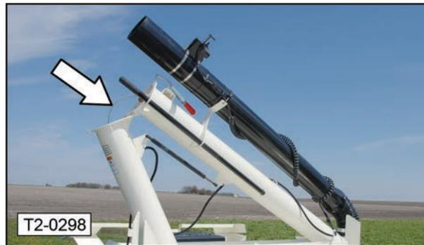
**Note:** On long-reach auger models, a spring loaded drive coupling will engage as soon as the auger begins to rotate. Refer to Section 8.3 for additional information.
