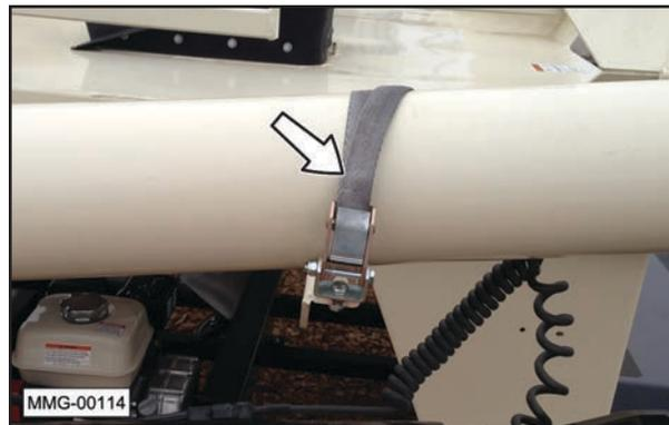
2. Open the upper tube and lock it in place with over-center clamp (3).
