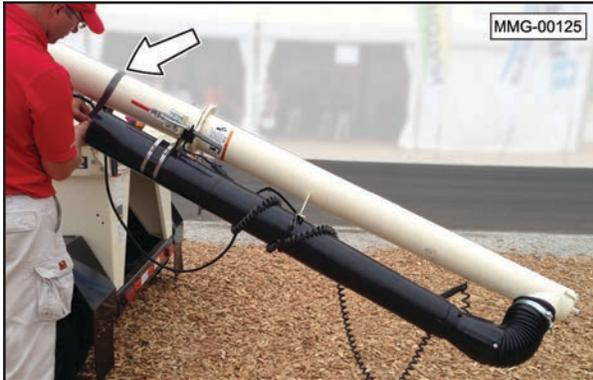
4. Remove the rubber retainer strap from the three-tier spout.
