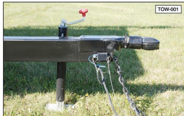
3. Remove the retainer pin. Release or open the receiver by pulling the locking cover back, as shown.
