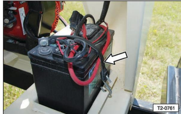
2. The battery is not charged when the engine is operating. If the battery is not charging using an external charger, check the fuse. Replace the fuse if necessary.
