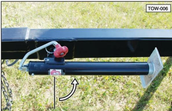
7. Close the receiver by pulling the spring loaded locking collar back to release the hitch mechanism. Install the retainer clip to prevent unwanted opening of the receiver.
