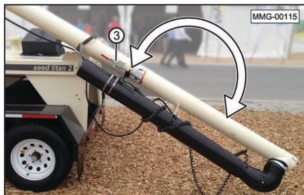
3. Release the retainer strap on the middle section of the conveyor tube.
