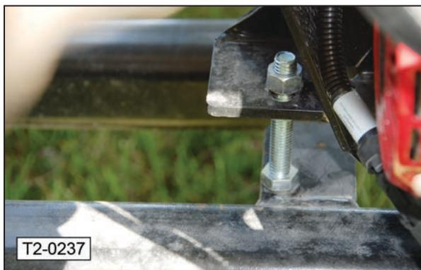
3. Loosen the jam nut on engine base adjusting bolt (2) and move the engine base to set the desired belt tension.
