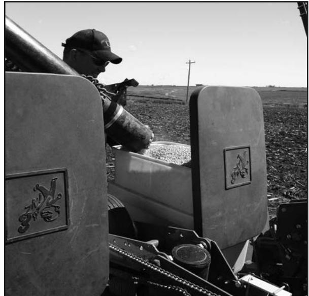
16. When the transfer of seed is complete, press the auger speed control switch to reduce the engine RPM and stop the auger.
