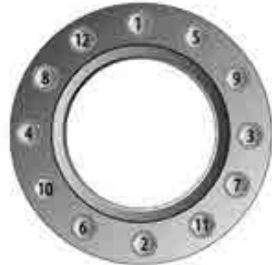
Fig 26 - 12 Bolt sequence
