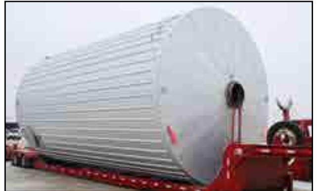
Fig 17 - Insulation and Galvalume Cladding:
