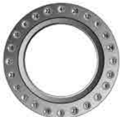
Fig 29 - 24 Bolt sequence
