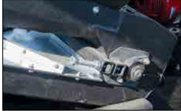
Fig 49 - Idler roller tension bolt at the bottom of belt
