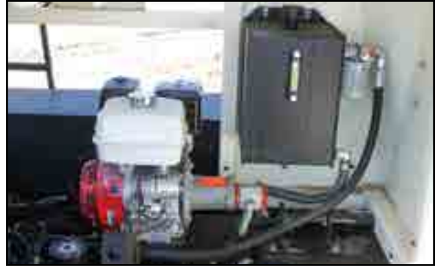
Fig 45 - Engine and hydraulic reservoir
