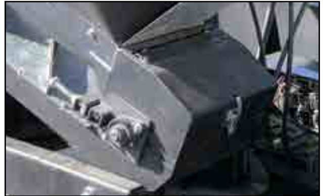
Fig 41 - Conveyor tube access door
