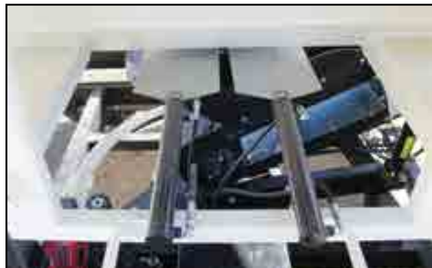
Fig 10 - Compartment slide gates
