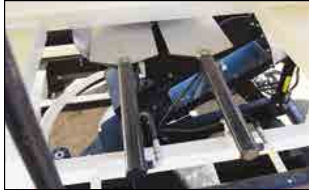
Fig 31 - Compartment slide gates
