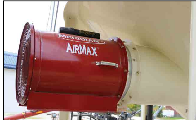
Fig 22 - AirMax™ In-Line fan
