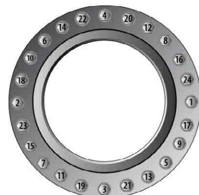
Fig 37 - 24 Bolt sequence
