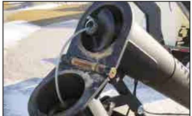
Fig 35 - Auger drive coupling
