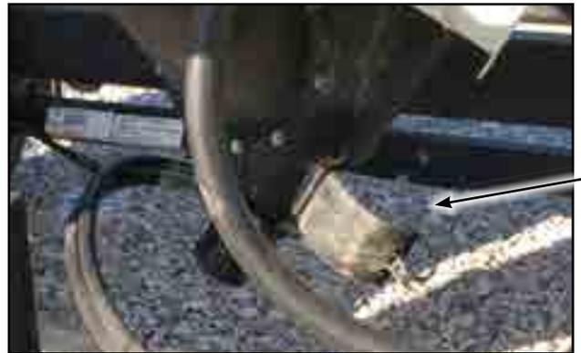
Fig 48 - Bottom clean-out access door
