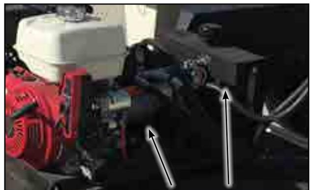
Fig 7 - Hydraulic pump and oil reservoir
