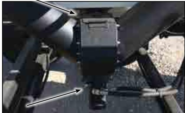
Fig 10 - Hydraulic auger motor and auger clean-out access
