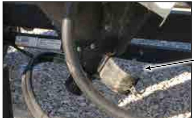
Fig 39 - Bottom clean-out access door
