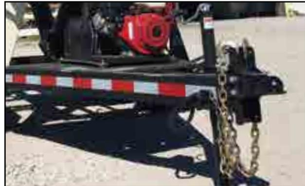
Fig 23 - Hitch receiver
