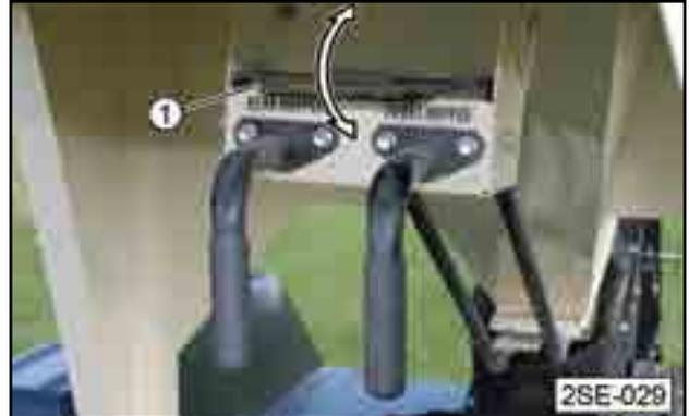
Fig 51 - Lift lock plate to use slide gate handles
