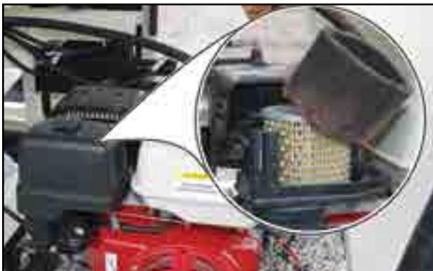
Fig 57 - Engine air filter
