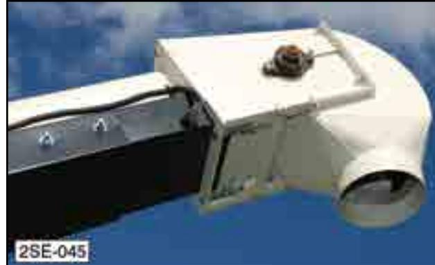
Fig 17 - Conveyor delivery spout
