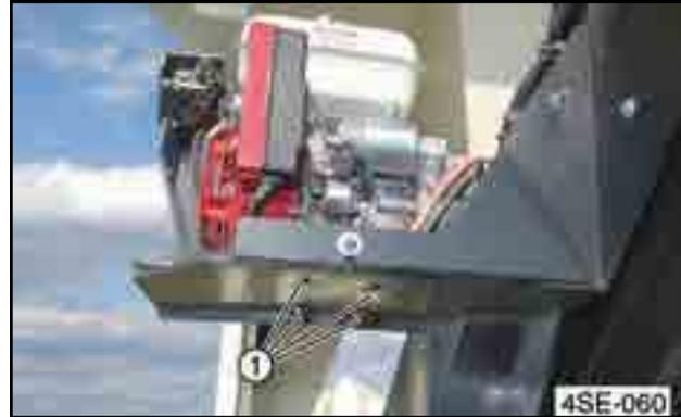
Fig 66 - Titan 4SE engine mount bolts
