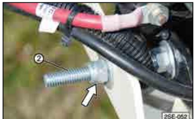
Fig 65 - Engine base adjusting bolt
