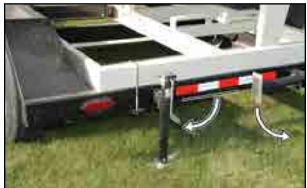
Fig 44 - Lower jacks when conveyor is at the rear
