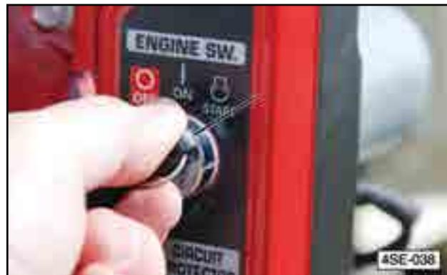
Fig 49 - Start the engine
