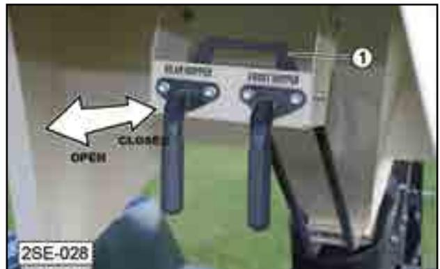
Fig 52 - Lock plate in "locked/closed" position
