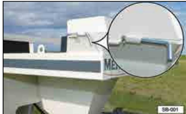
Fig 32 - Lock-down arm and latch pin
