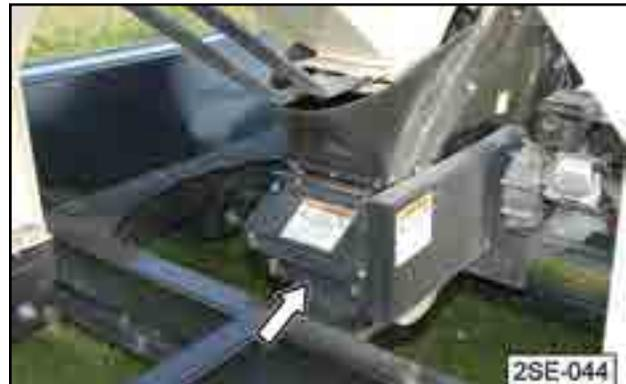
Fig 77 - Conveyor tube access door
