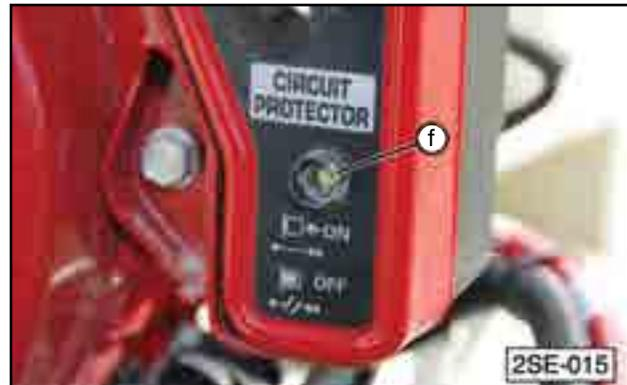
Fig 9 - Engine Circuit Protector
