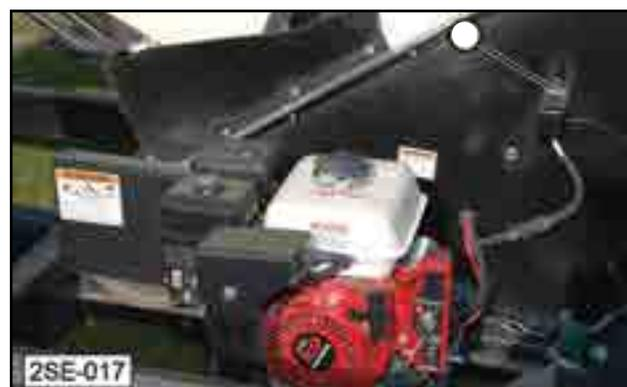
Fig 12 - Throttle Switch
