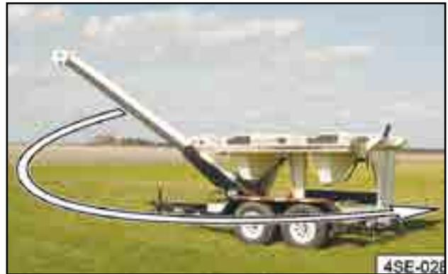
Fig 46 - 4SE tube shuttle and swing
