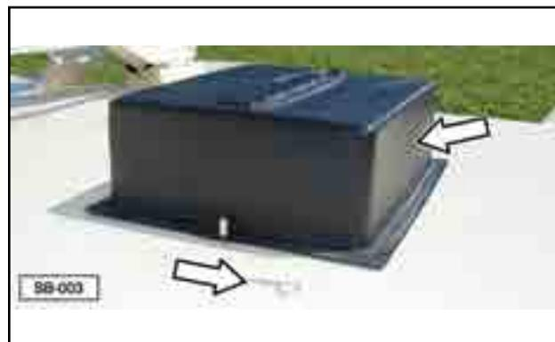
Fig 34 - Remove protective chute cover
