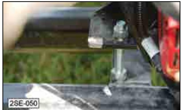
Fig 64 - 2SE Engine base stabilizing bolts
