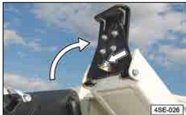
Fig 42 - Raise Titan 4SE lock plate
