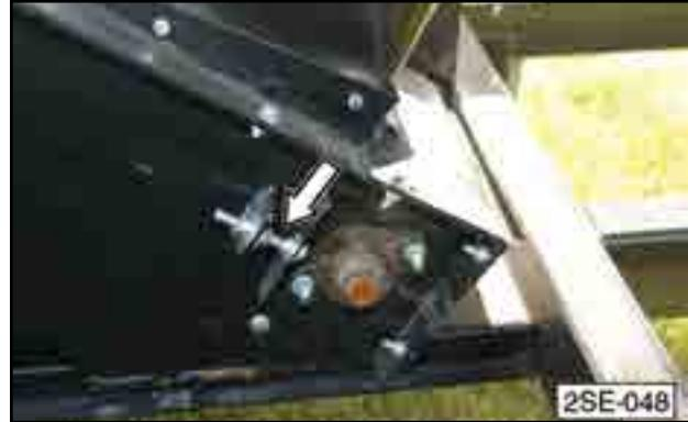
Fig 71 - Conveyor belt tension bolt
