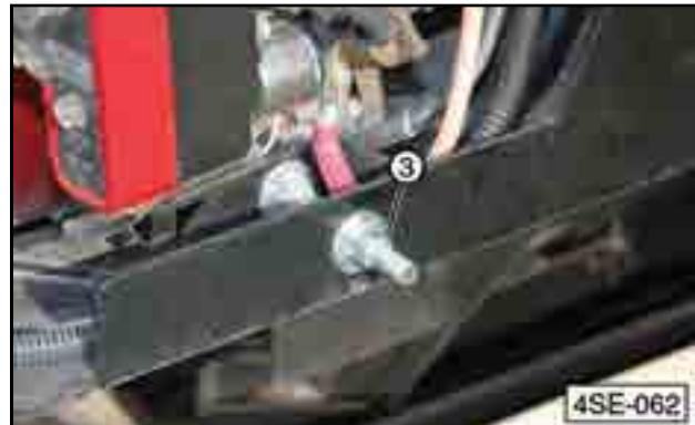
Fig 68 - 4SE engine base adjusting bolt
