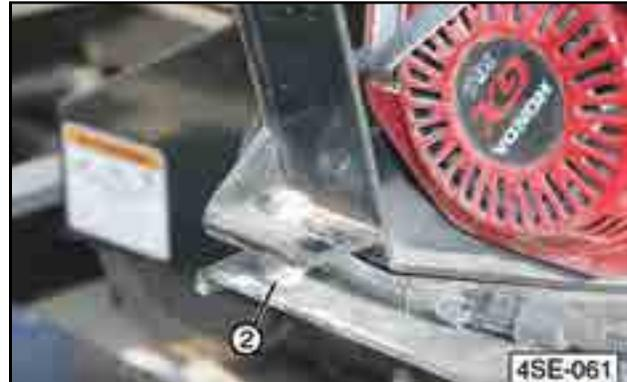
Fig 67 - Titan 4SE engine base stabilizing bolts
