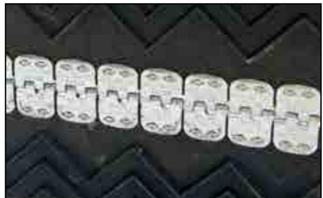
Fig 75 - Conveyor belt lacing
