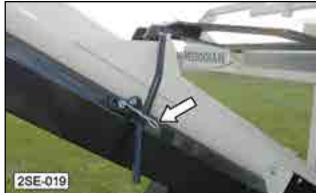
Fig 39 - Lock plate handle on Titan 2SE
