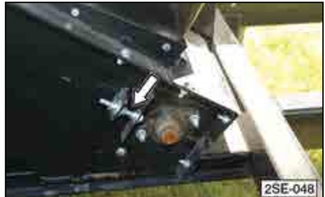
Fig 74 - Belt Tension bolts
