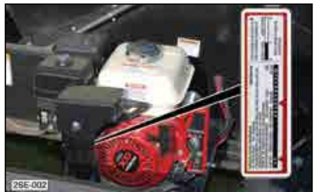
Fig 2 - Serial number on engine
