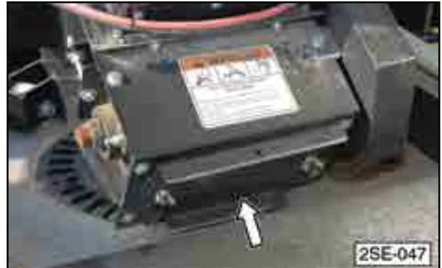
Fig 73 - Conveyor tube access door
