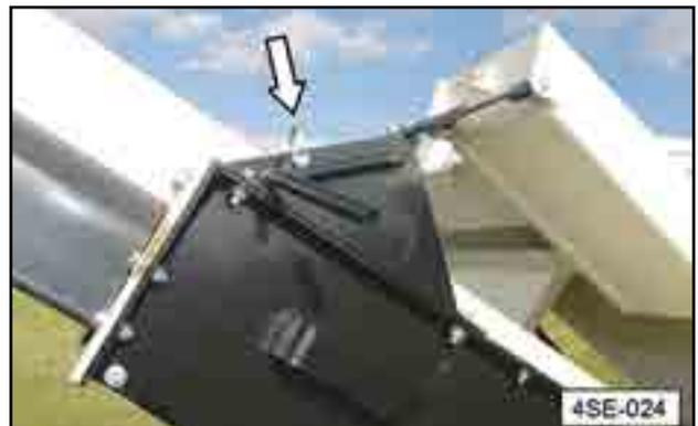
Fig 14 - Conveyor tube transport lock
