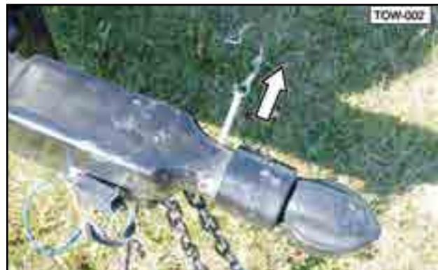
Fig 25 - Hitch receiver Retainer pin
