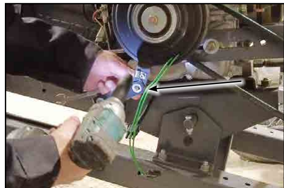
Fig 3 - Disconnect rubber link from clutch
