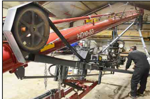
Fig 4 - Open gearbox belt guard
