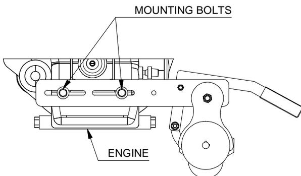
After installing the engine pump drive pulley, the belt (BX-38) can be installed. Provide slight tension to the two mounting bolts, pull back on the pump bracket and then tighten the mounting bolts. This step may need to be repeated until proper belt tension is attained. Preferred tension is 20lbs pull per 1/4" belt deflection. Install the belt guard.
