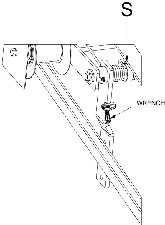
There is also an adjustment to be made on the spring if more spring tension is required. Spring adjustment is done by loosening the square headed set screw "S" on the shaft collar. With the belts out of the way from the pulley, lower the pulley down allowing the spring to move down and retighten the set screw. Lift pulley up and place belts back under the pulley and test for required tightness.
