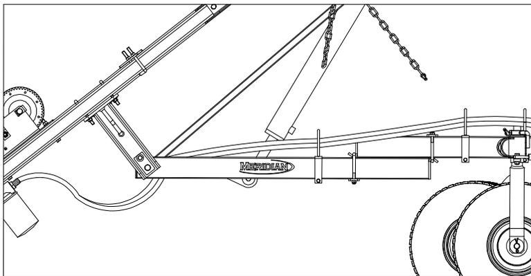
Run the hoses through the three hose rings along the expandable frames and zip tie hoses to the frames. Leave a significant curve in the hoses just below the main frame anchor.
