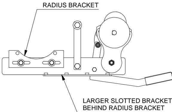
The big block pump has a small radius mounted stationary bracket that bolts on with two 7/16" x 1-1/2" bolts. It has a larger slotted bracket fastened to the back side of the stationary bracket which allows belt tensioning.
