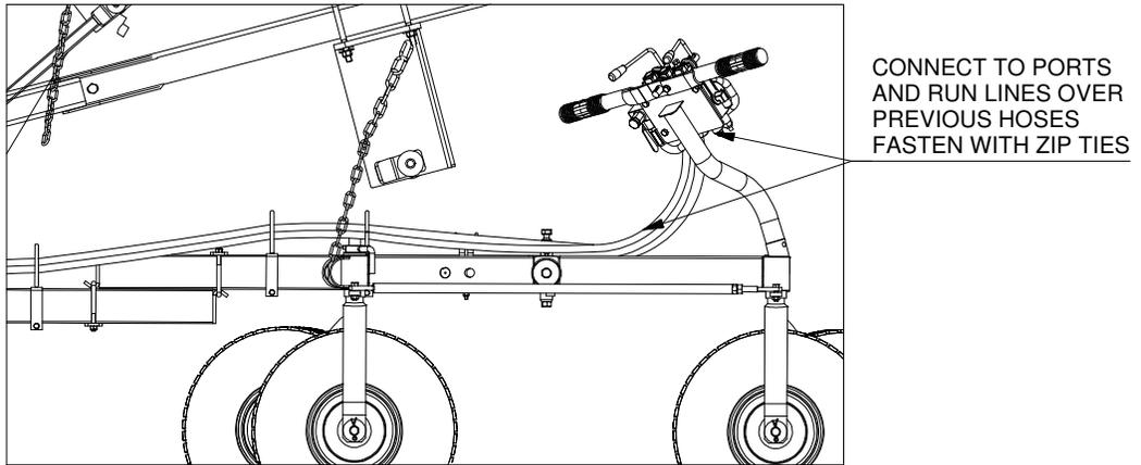
Connect the #8 hose to the "T" fitting on the winch motor and the #7 hose to the fitting on the silver relief valve block.
