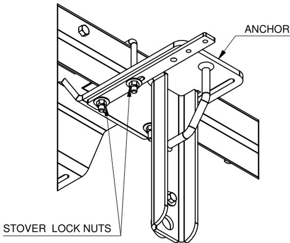
Secure filter mounting bracket to bottom of Anchor using the 3/8" Stover lock nuts.
