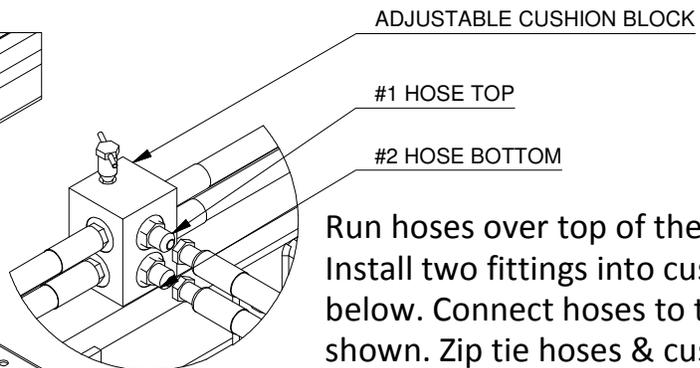
Run hoses over top of the tank brackets. Install two fittings into cushion block as below. Connect hoses to the fittings as shown. Zip tie hoses & cushion block to the frame.
