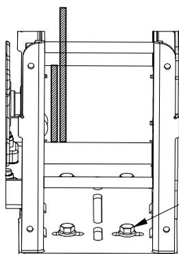
INSTALL FLANGED BOLTS FROM THE TOP DOWN WITH THE NUTS AT THE BOTTOM
