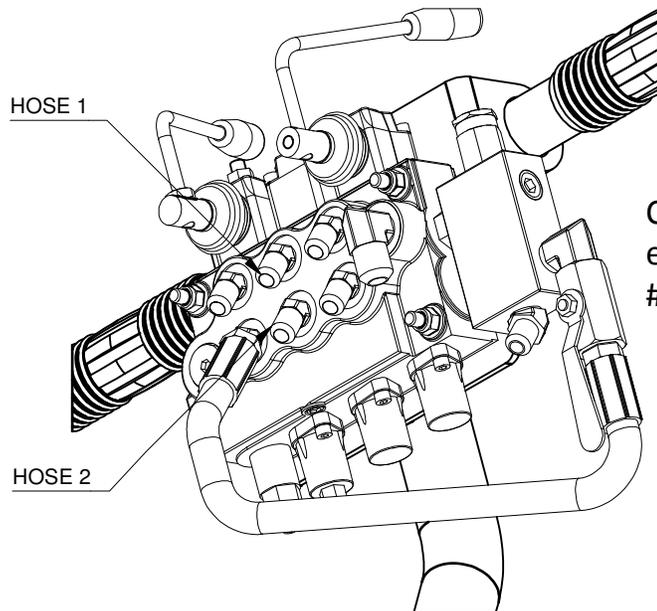
Connect #2 hose first and then #1 to ease installation as it is below fitting #1.
