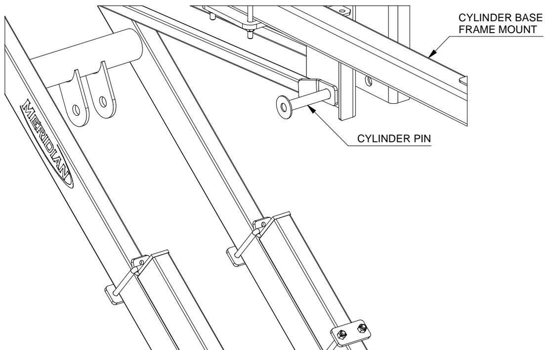
Install base end of the hydraulic cylinder into the Cylinder Base. Note the position of the hydraulic cylinder fitting ports. Push the 3/4" X 5" cylinder pin through the cylinder pin boss and the other side of the Cylinder Base. Install the 3/4" SAE washer and 3/16" X 1-1/2" cotter pin to retain the cylinder pin. Securely tighten all the U-bolts and lock nuts on the Cylinder Base.
