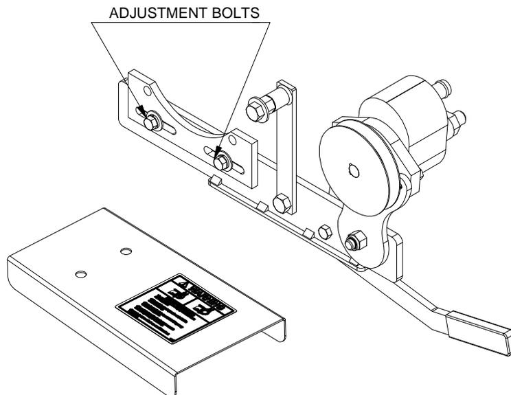
After installing the drive pulley, the belt (BX-34) can be installed. Provide slight tension to the two 3/8" adjustment bolts at the bottom of the radius bracket. Pull back on the pump bracket, tightening the adjustment bolts. This step may be repeated until proper belt tension is attained. Preferred tension is 20lbs per 1/4" belt deflection. Install the belt guard.
