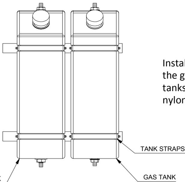
Install the hydraulic oil tank to the inside and the gas tank to the outside. Fasten down the tanks with the four tank straps and 5/16" nylon lock nuts.
