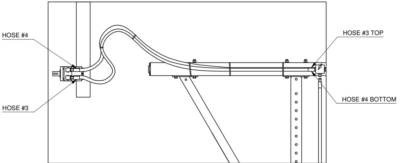
Install two drive motor fittings onto each of the drive motors. Then install the #3 and #4 hoses into the cushion block as shown above. Now run the hoses along the axle to the left and shape hoses into an "S" shape and hook up to the LH drive motor ports as designated.
