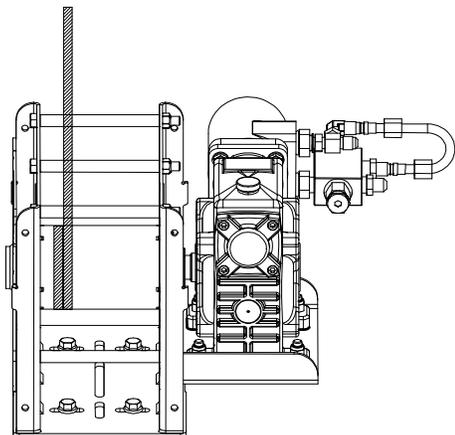
Secure the winch to the winch plate with three 3/8" x 3/4" flanged bolts and 3/8" flanged nuts.
