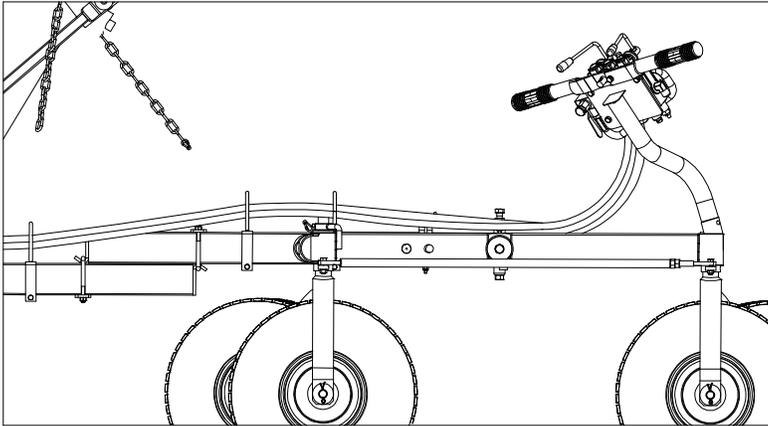
Run the two drive circuit hoses #1 & #2 down from the valve so they have a large curve with a slight sag at the curve. Run hoses along over the transport bar.
