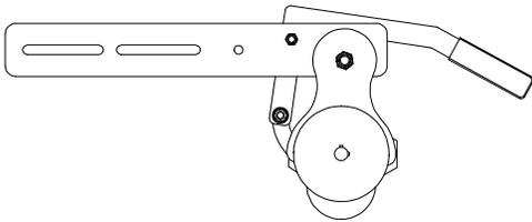
The pump has a slotted bracket that bolts directly to the engine with two 7/16" x 1-1/2" bolts. The entire assembly slides to aid in tensioning the pump belt.
