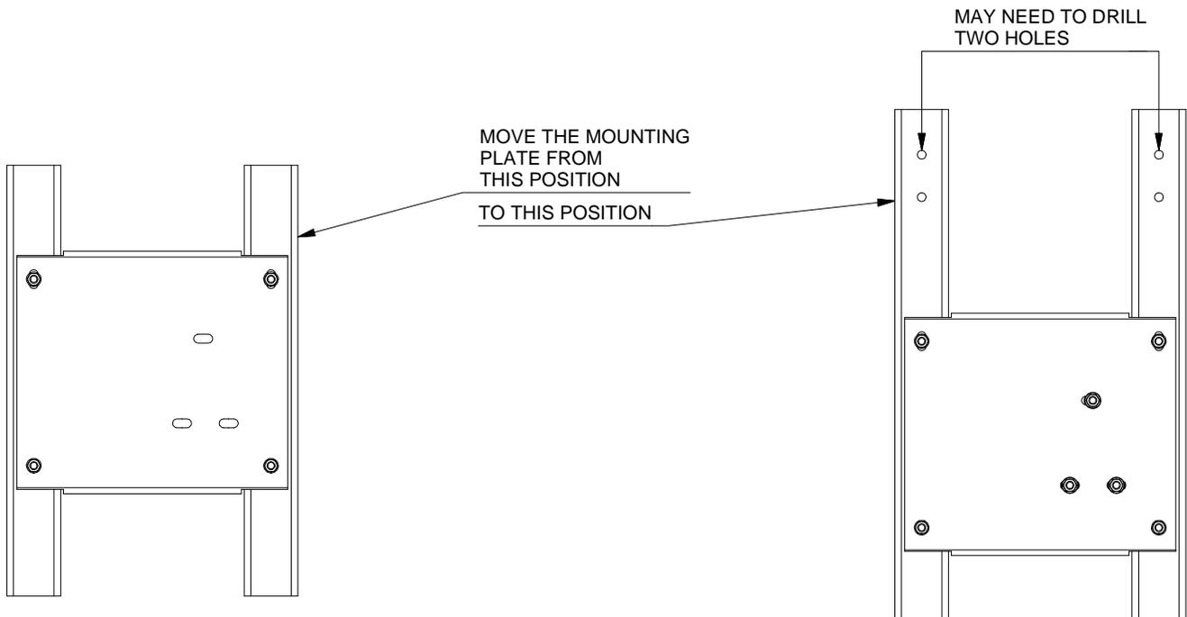
**Cable Roller Bracket Assembly for 33'**
