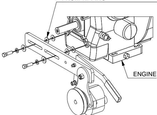
To mount the pump, first install a 7/16" lock washer and 7/16" flat washer onto the 7/16" x 1-1/2" bolt. Insert the bolt through the slotted bracket, then install two 3/8" flat washers onto the bolt and insert into the 7/16" engine block mounting holes. Note: there are four 3/8" completely round flat washers to be used on the Vanguard engines. There are four 3/8" flat washers that are nipped off on the edge to fit the Kohler engines.
