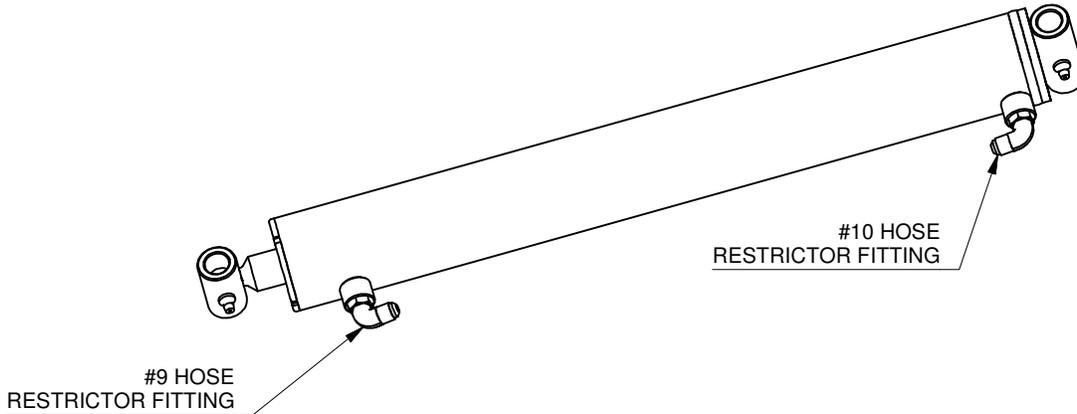
Connect #9 hose to the rod end of cylinder and the #10 hose to the base end of the cylinder.
