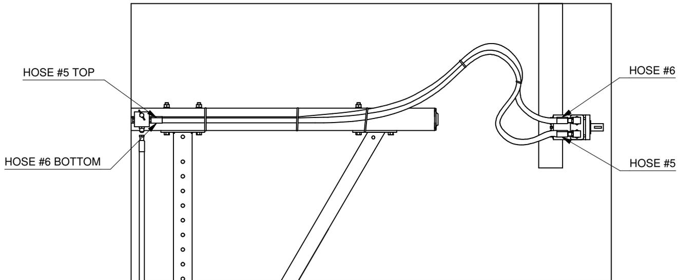
Install the #5 and #6 hoses into the cushion block as shown above. Now run the hoses along the axle to the right and shape hoses into an "S" shape and hook up to the RH drive motor ports as designated.
