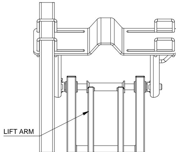
Secure Frame Pin with  $\frac{5}{16}$ " X 1" - NC bolt and  $\frac{5}{16}$ " spring washer.
