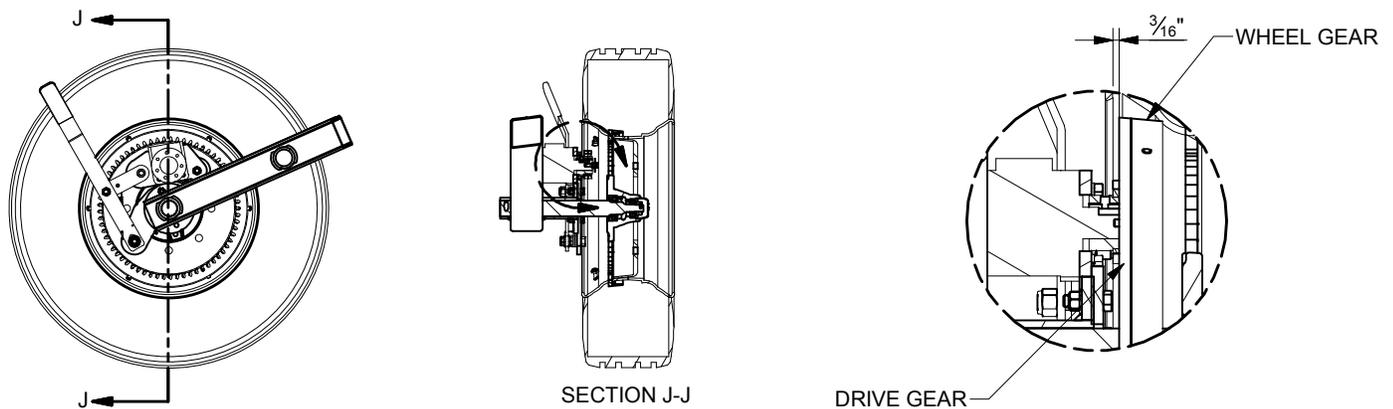
Once welding is complete, recheck gear engagement. If more engagement is required, the outer 1/2" flange nut can be loosened at the bottom of the handle. The 1" slot in the bottom of the handle will allow the handle to be lifted up which will mesh the drive gear deeper into the wheel gear.
