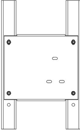
Use the set of holes which position the plate closest to the intake.
