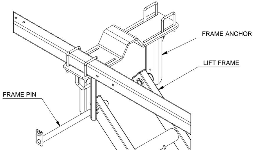
Install the Lift Arm between the Lift Frame and slide the Frame Pin all the way through.
