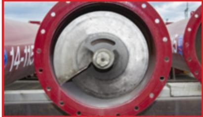
Fastened Spline and Hub Connection
