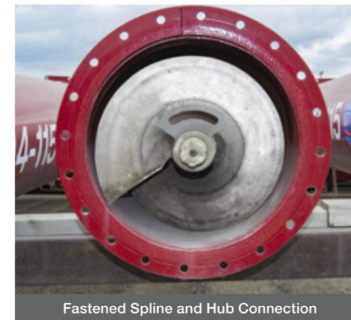
Fastened Spline and Hub Connection
