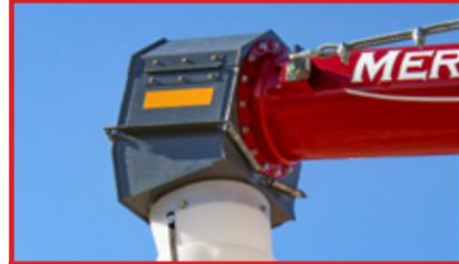
Patented Spring Loaded Blow Out Doors
