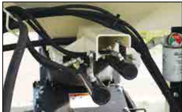
Fig 11 - Compartment slide gate cylinders
