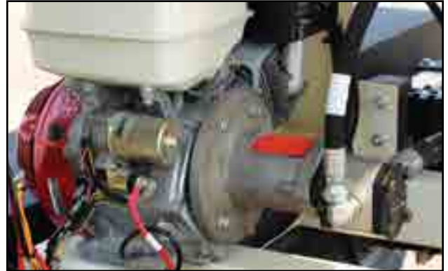
Fig 54 - Engine and hydraulic pump
