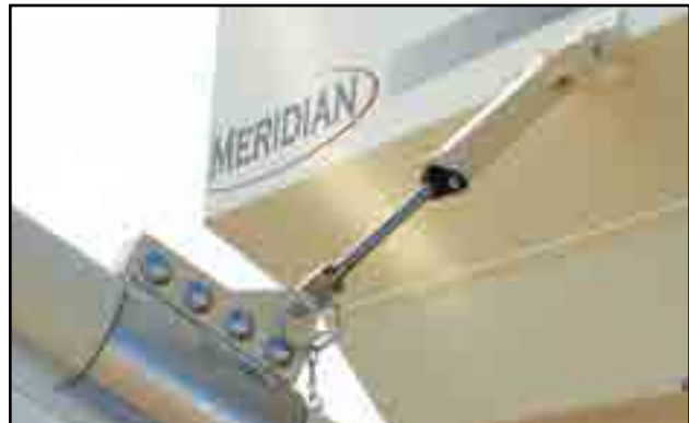
Fig 10 - Conveyor tube damper mechanism and transport lock
