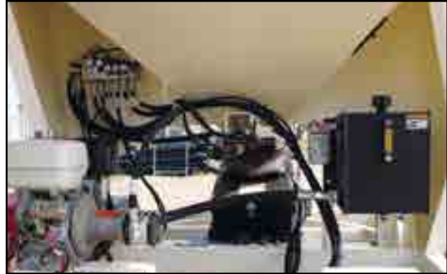
Fig 8 - Engine, hydraulic oil reservoir and filter
