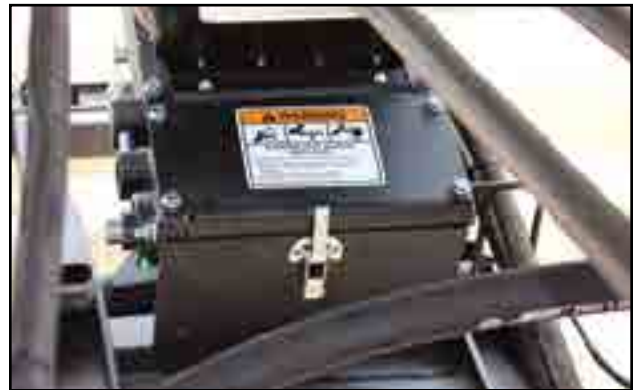
Fig 48 - Conveyor tube access door
