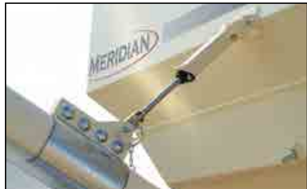
Fig 26 - Conveyor tube transport lock w/ damper mechanism
