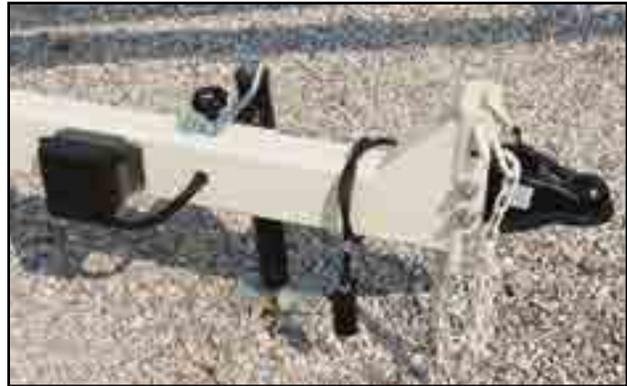
Fig 50 - Break-Away system control box
