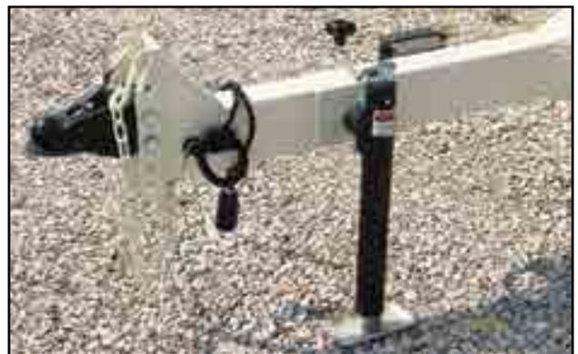
Fig 20 - Trailer hitch with safety chains
