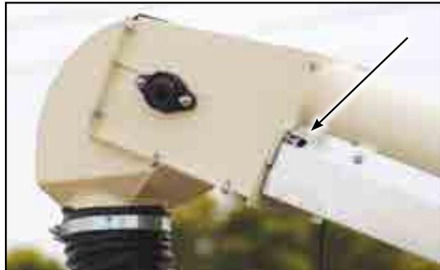
Fig 45 - Discharge roller adjustment bolt, one on each side
