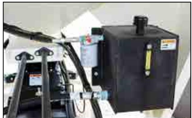
Fig 7 - Hydraulic reservoir and filter
