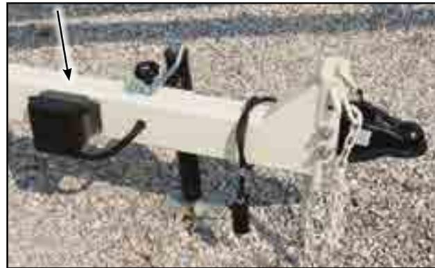
Fig 16 - Break-Away system control box
