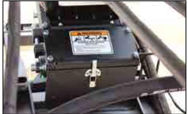
Fig 36 - Conveyor tube access door
