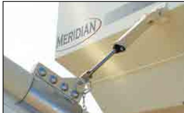
Fig 10 - Tube transport Lock and damper mechanism
