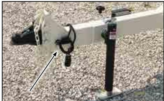
Fig 51 - Break-Away cable on hitch tongue
