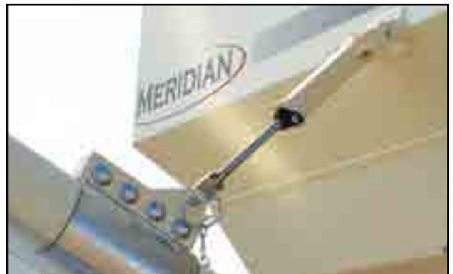
Fig 30 - Conveyor tube transport lock and damper mechanism
