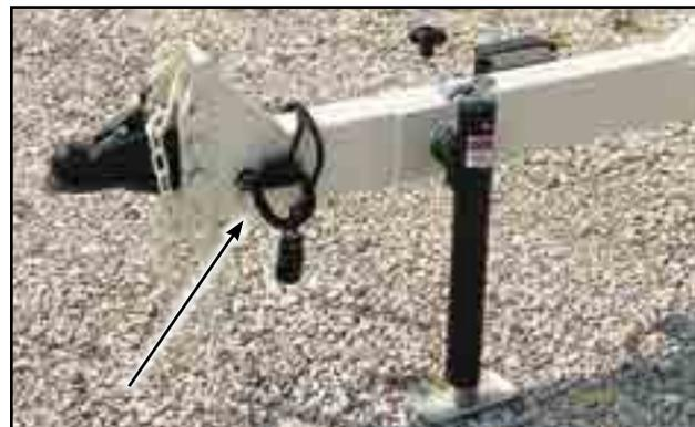
Fig 17 - Break-Away cable on hitch tongue
