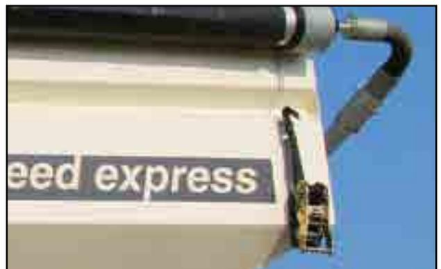
Fig 25 - Tarp tension ratchet straps
