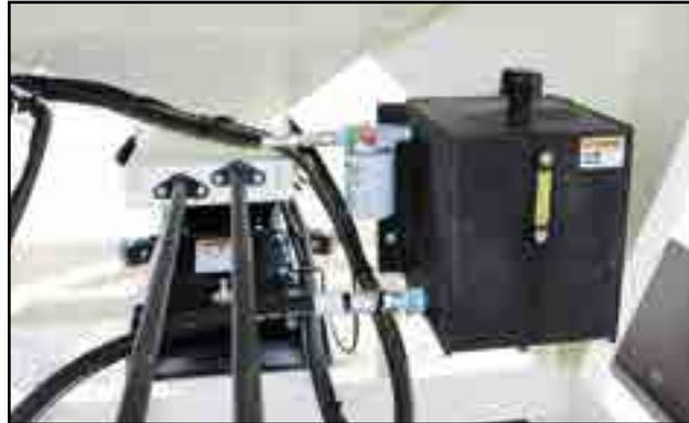
Fig 40 - Hydraulic oil reservoir and filter
