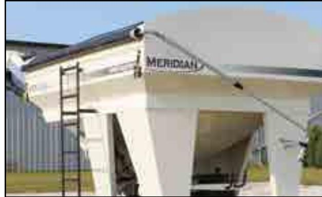
Fig 15 - Roll tarp and crank handle
