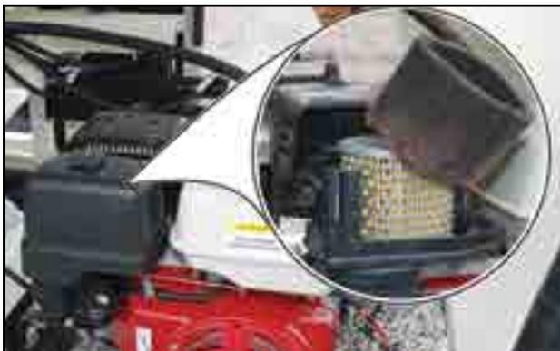
Fig 37 - Engine air filter
