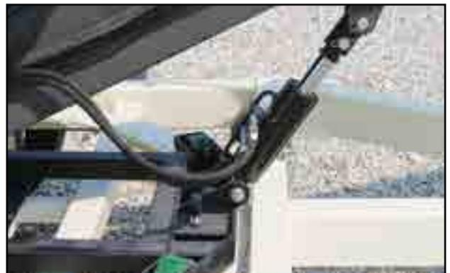
Fig 31 - Conveyor turret assembly and pivot platform
