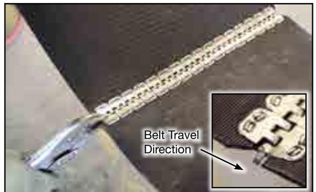
Fig 48 - Crimp lacing and taper belt corner
