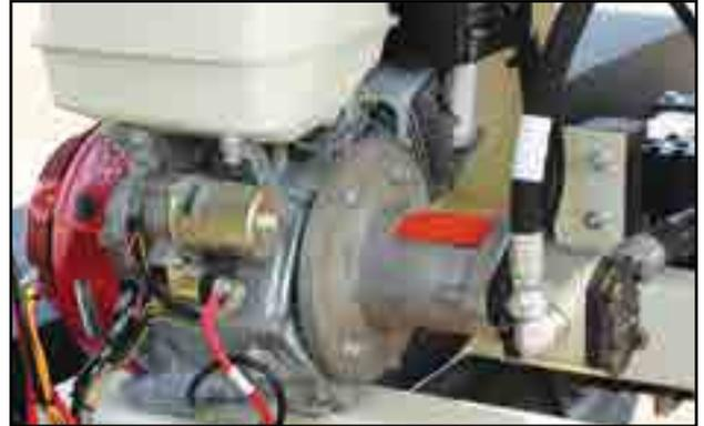
Fig 42 - Engine and hydraulic pump
