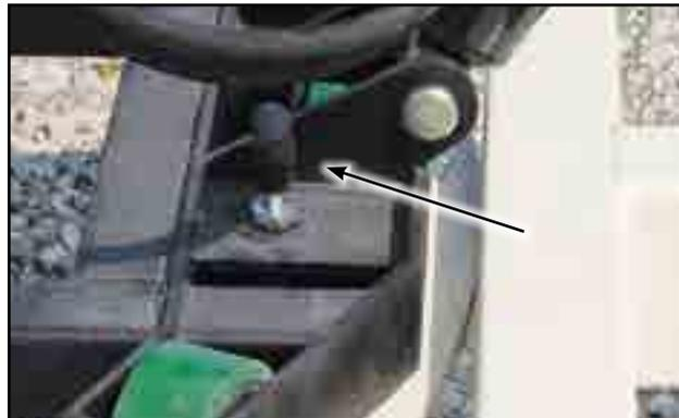
Fig 33 - Turret assembly locking plunger pin
