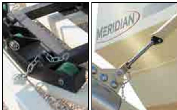
Fig 35 - Secure conveyor tube for transport
