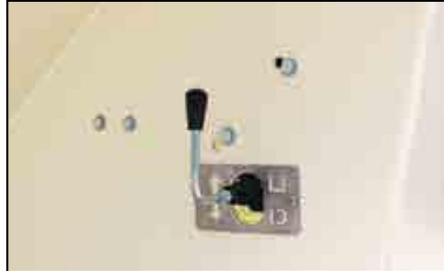
Fig 8 - Hydraulic valve lever
