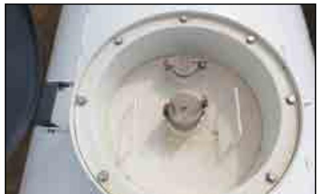
Fig 19 - Inside the Spill Box on standard tank
