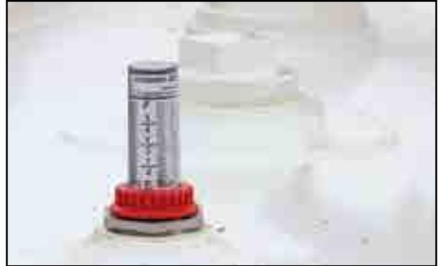
Fig 8 - Liquid level gauge
