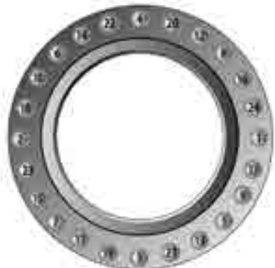
Fig 29 - 24 Bolt sequence
