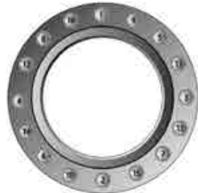
Fig 27 - 16 Bolt sequence
