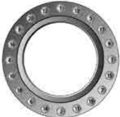
Fig 28 - 20 Bolt sequence
