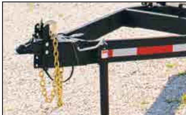
Fig 21 - Trailer hitch with safety chains
