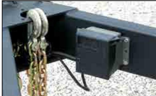
Fig 16 - Break-Away system control box
