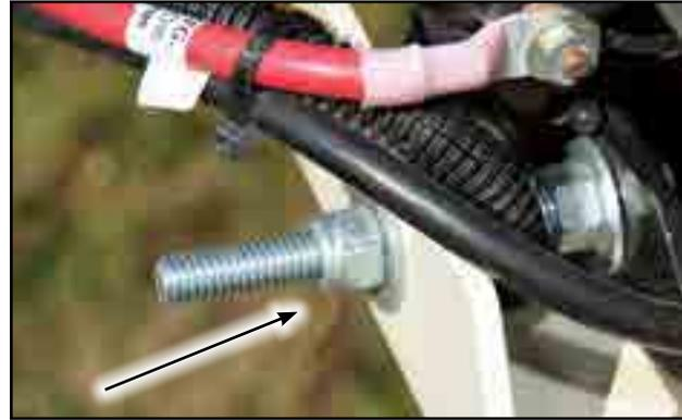
Fig 47 - Engine base adjustment bolt
