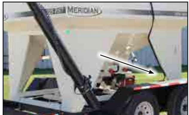
Fig 8 - Battery in corner of frame
