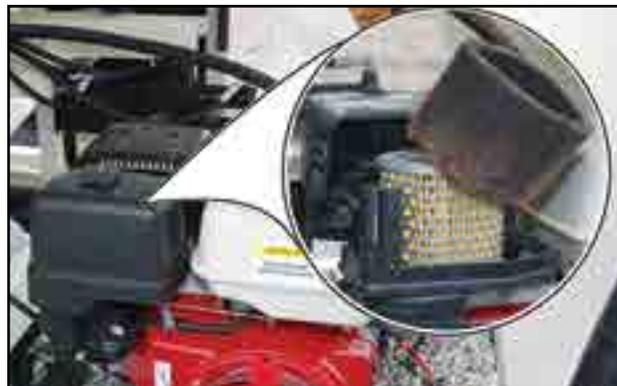
Fig 39 - Engine air filter
