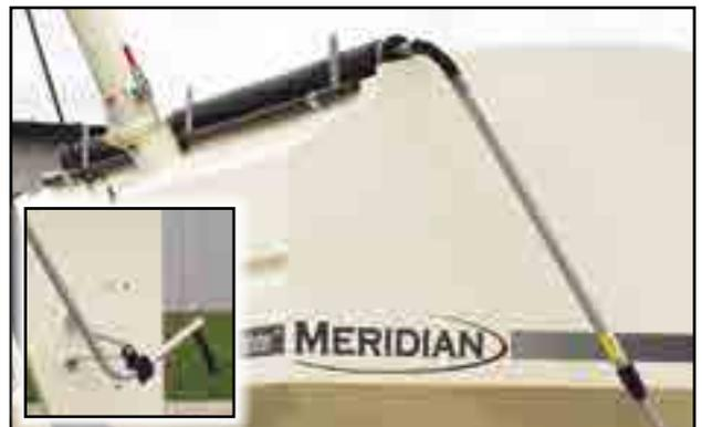
Fig 14 - 225 RST Roll tarp and crank handle
