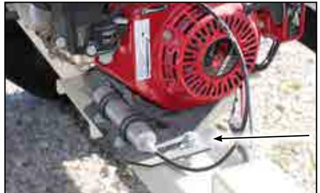
Fig 50 - Engine base stabilizing bolt
