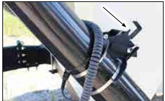
Fig 37 - Actuator toggle switch on delivery spout
