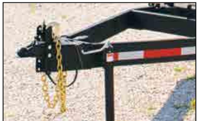
Fig 15 - Tongue on the bumper hitch trailer
