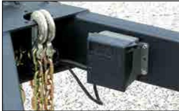
Fig 52 - Break-Away system control box
