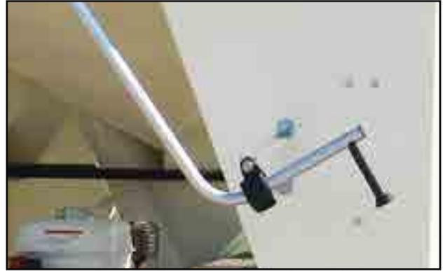
Fig 27 - Remove tarp crank handle
