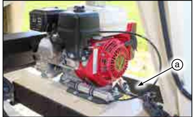
Fig 43 - Actuator to engine wiring harness
