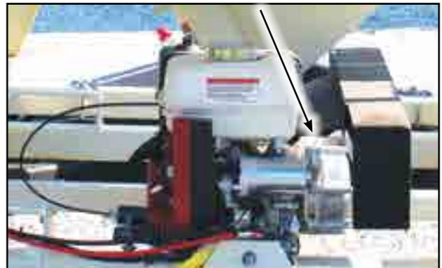
Fig 7 - Centrifugal clutch and auger drive belt
