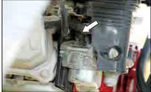
Fig 42 - Engine speed setscrew
