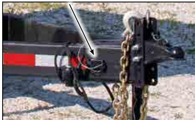
Fig 53 - Break-Away cable on hitch tongue
