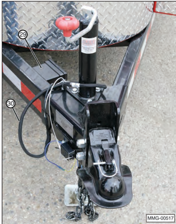
(29) Breakaway brake system. (30) Wiring harness with 7-pin automotive connector.
