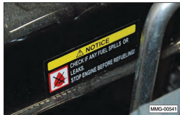
7. Safety Decal on Option Air Compressor/Welder Unit (contact OEM supplier for replacement).
