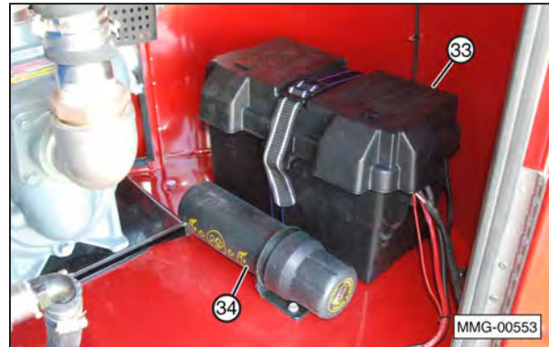
(33) Battery box. (34) Literature tube.
