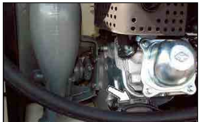
Fig 2 - Engine serial number location
