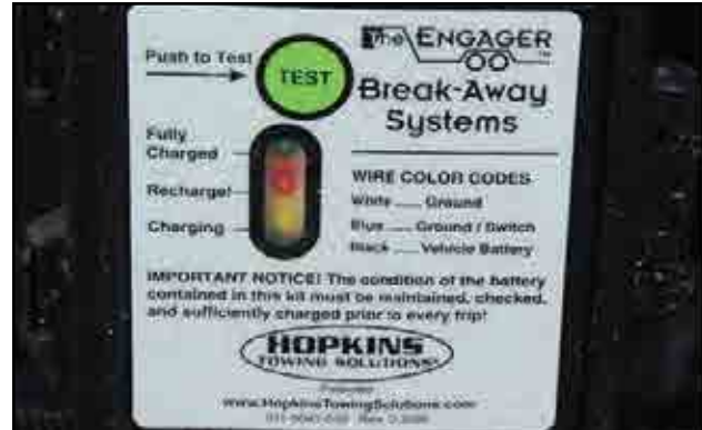
Fig 65 - Trailer Break-Away System
