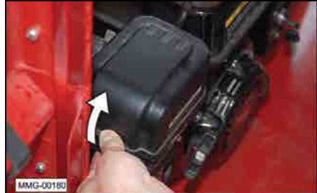
Fig 60 - Air filter cover
