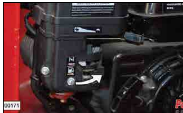
Fig 44 - Engine fuel lever
