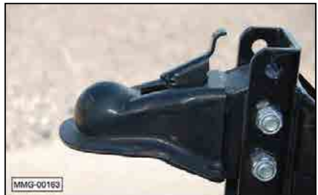
Fig 29 - Ball hitch receiver
