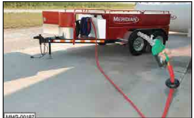
Fig 38 - Extend hose for fueling
