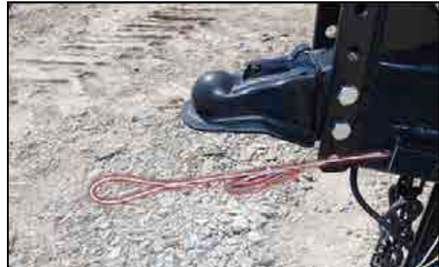
Fig 66 - Break-Away switch and pin
