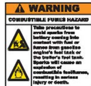
Fig 8 - Safety decals inside driver's side compartment door
