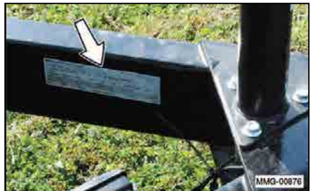
Fig 1 - Trailer VIN number location
