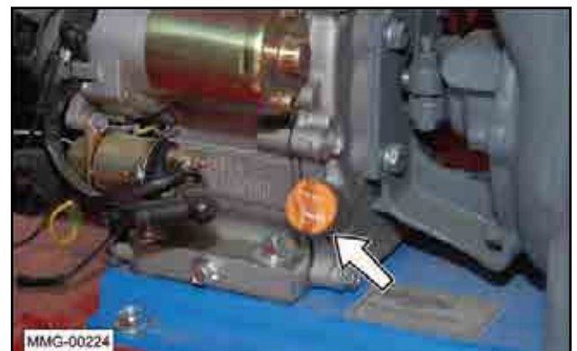
Fig 59 - Engine oil plug
