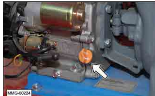
Fig 5 - Engine serial number location
