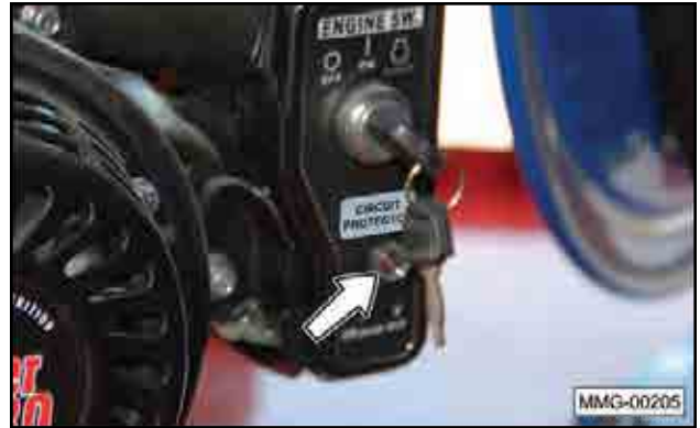
Fig 63 - Engine circuit protector
