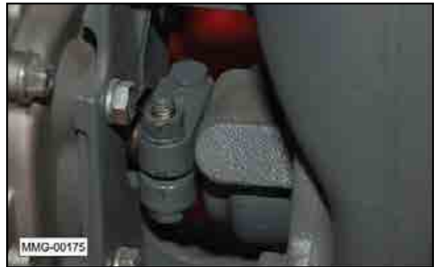
Fig 64 - Engine circuit protector
