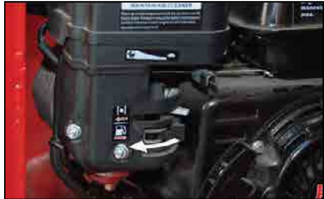
Fig 49 - Fuel valve under front of trailer
