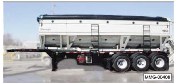
3. Position the tractor in a straight line in front of the trailer, fifth wheel to trailer kingpin.
