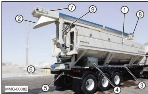
(1) Seed Compartments. (2) Hopper. (3) Seed Tender Frame. (4) Control Panel and Wireless Remote Control (not shown). (5) Trailer. (6) Underbin Conveyor. (7) Incline Conveyor in Transport Position. (8) Delivery Spout. (9) Pivot Frame.
