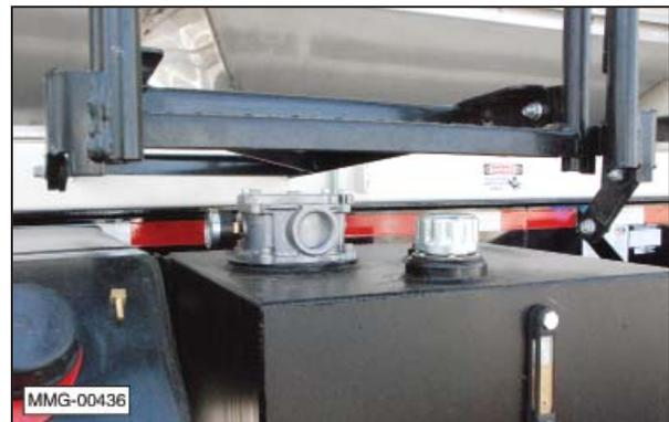
Annually, a sample of hydraulic oil should be taken to a dealer with oil analysis capability. When analysis shows the need to change the oil, use the following procedure. Use an AW HVI Hydraulic ISO 32 oil.
