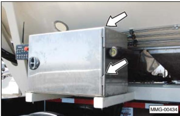
The hydraulic manifold enclosure box door hinges are equipped with grease zerks.
