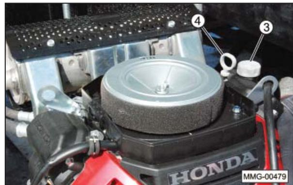
11. Run the engine for one minute and recheck the oil level. Add oil, as needed, to reach the upper limit mark on the dipstick.
