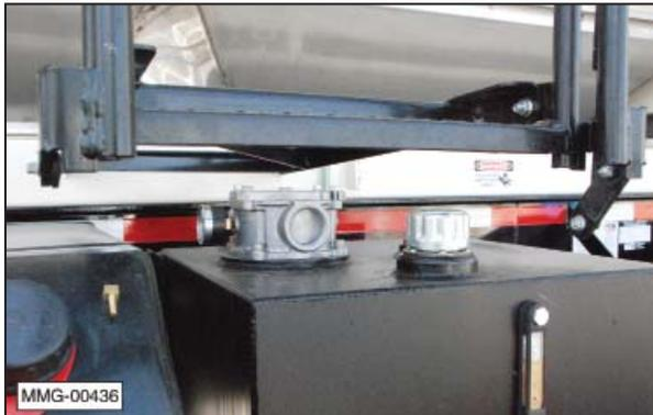
A hydraulic oil filter change is recommended annually or every 400 hours of operation, or whenever the oil filter flow gauge indicates the need for a filter change.
