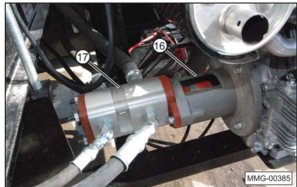
(16) Coupling (Engine to Pumps). (17) Hydraulic Pumps.
