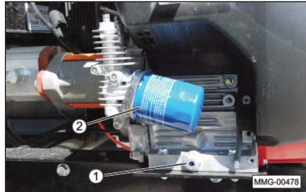
6. Reinstall the engine drain plug with a new sealing washer and tighten.
