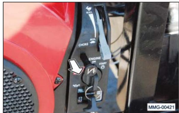
3. Move the throttle lever about 1/3 of the way to the MAX position.
