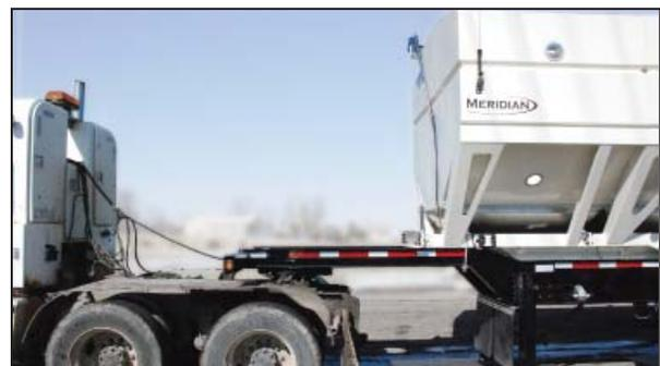
5. Test the integrity of the coupling by putting the semi in first gear and moving forward no more than six inches.
