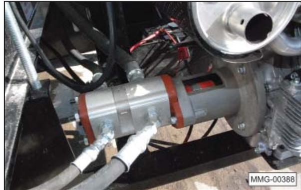
1. Remove the two pump mounting bolts.
