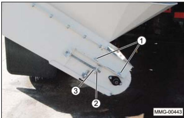
3. Loosen locknuts (2) on each side of the belt tension mechanism.
