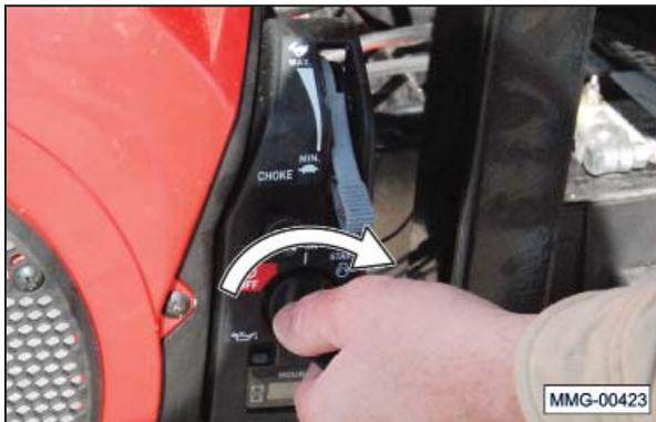
5. Warm up the engine for two or three minutes. If the choke knob was pulled out to start the engine, gradually push it in as the engine warms up.
