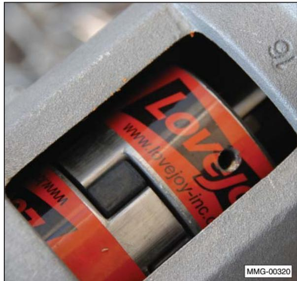
3. Loosen the setscrews in each coupling half and remove the old couplings. Install new couplings on the engine shaft and the pump shaft. When completely assembled, the shaft length in each coupling half should be the same. Tighten the pump end setscrews to 78 to 87 lb-in. Do not tighten the engine shaft coupling at this time.
