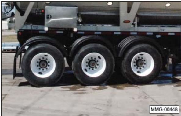
1. Initially check the wheel bolt torque at 50 miles and after each wheel removal.
