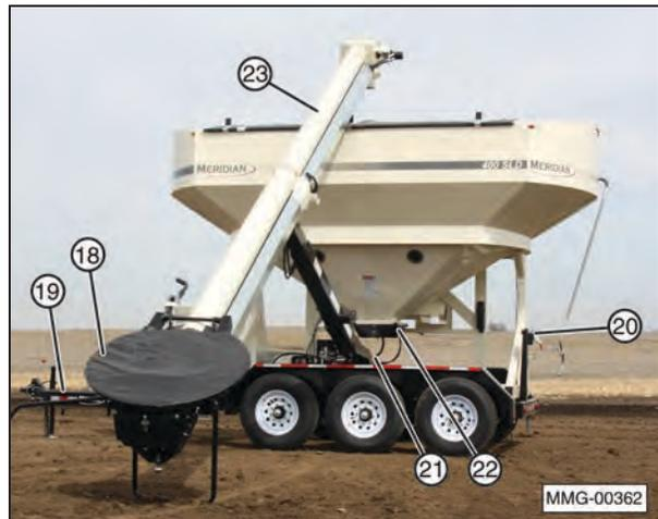
(18) Hopper and Cover. (19) Breakaway Trailer Brake System. (20) Transport Lock (Field and Road). (21) Pivot Platform. (22) Bin Slide Gates and Cylinders. (23) Conveyor in Self-loading Position.
