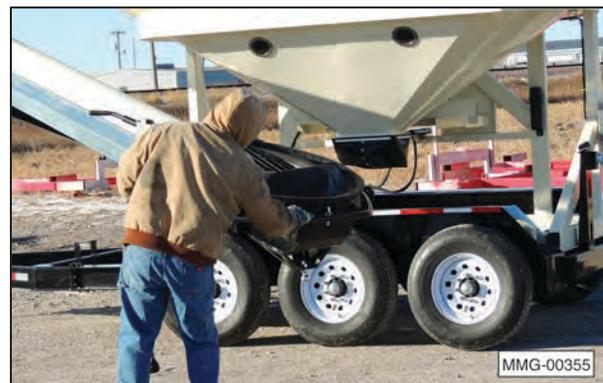
15. Use the conveyor left or the conveyor right buttons (switches) to position conveyor arm into the desired position. The photos show the self-filling position.
