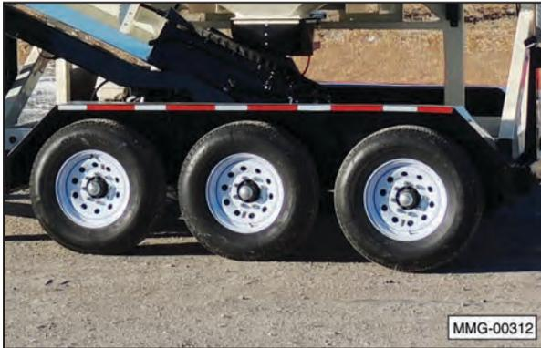
1. Initially check the wheel bolt torque at 5, 10, 25, and 50 miles and after each wheel removal.
