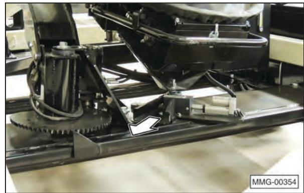
24. Press and hold the toggle switch upward to lock the ball coupling into the conveyor hitch receiver.
