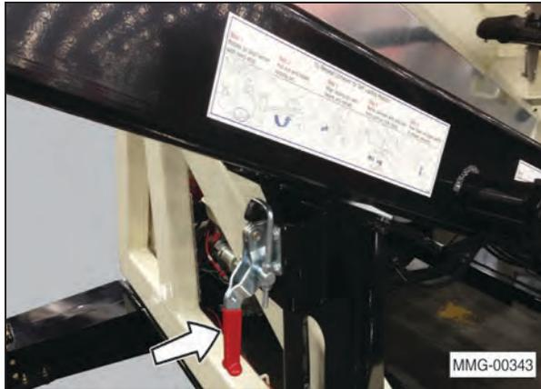
2. If not already removed, remove the protective cover from the seed pan. It may be necessary to lower the hopper in order to remove the cover. To lower the hopper, pull out on the sliding lock collar and raise the handle to lower the hopper.
