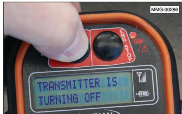
When the POWER button is pressed and held, the message "Transmitter is turning OFF" will be displayed.
