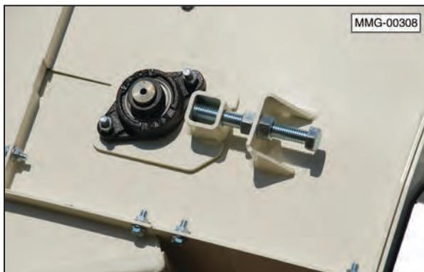
1. Loosen the locknuts on the adjusting bolt.
