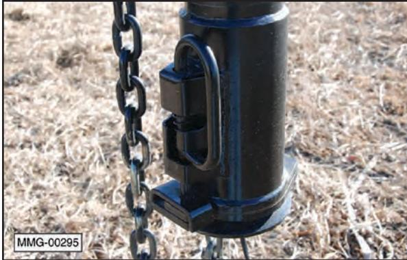
7. Position the trailer's coupler directly over the ball in the bed of the tow vehicle.
