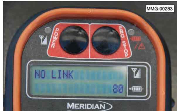
If the "NO LINK" message appears, the remote transmitter is not communicating with the control panel on the seed tender. Make sure the ON/OFF key switch is in the ON position.
