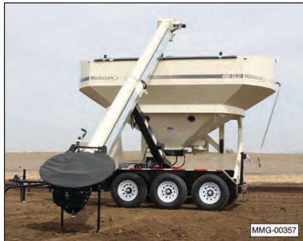
16. If desired, release the stand lock pin and rotate the stand downward. Engage the lock pin when the stand is fully extended.
