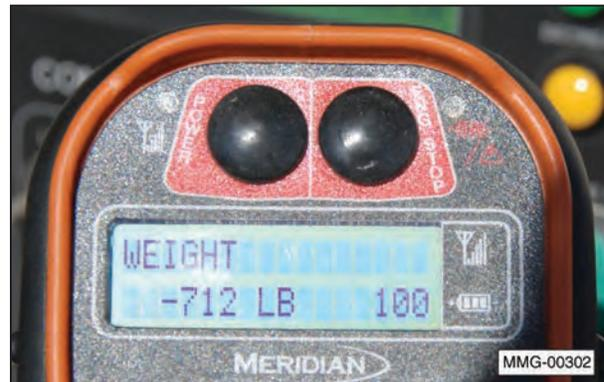
The remote transmitter will display the WEIGHT of the seed in the seed compartments in pounds. It also displays the battery life of the two AA batteries in a percentage of remaining life.
