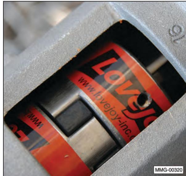
4. Loosen the setscrews in each coupling half and remove the old couplings. Install new couplings on the engine shaft and the pump shaft. When completely assembled, the shaft length in each coupling half should be the same. Tighten the pump end setscrews to 78 to 87 lb-in. Do not tighten the engine shaft coupling at this time.
