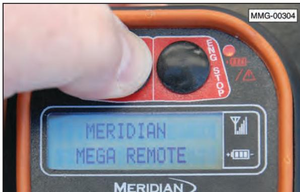
Pressing the POWER button turns the remote transmitter ON and displays the message "Meridian Mega Remote".
