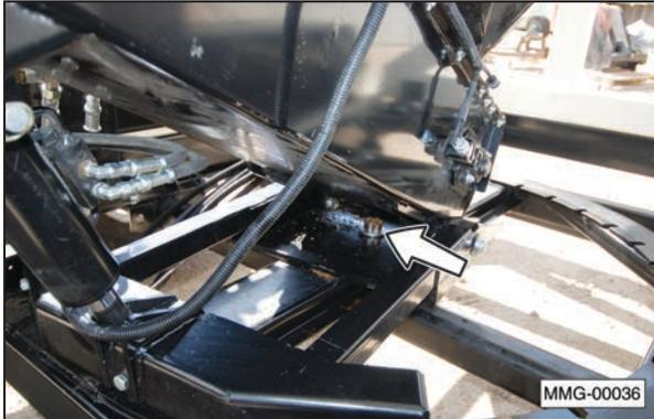
4. Make sure the tarp roll up cable is tensioned correctly. Refer to the OEM manual for additional information.
