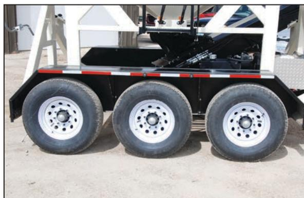
1. Initially check the wheel bolt torque at 10, 25, and 50 miles and after each wheel removal. Refer to the Wheel Bolt Torque Requirements section in this manual for tightening instructions.
