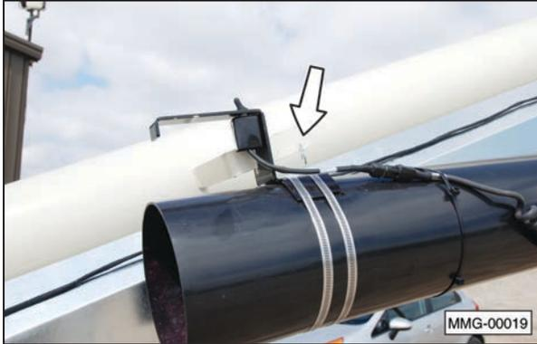
8. Manually rotate (pull or push) the conveyor to place the delivery spout over the planter.
