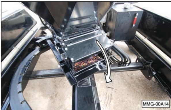
2. Position the crimped belt fastener in the opening.
