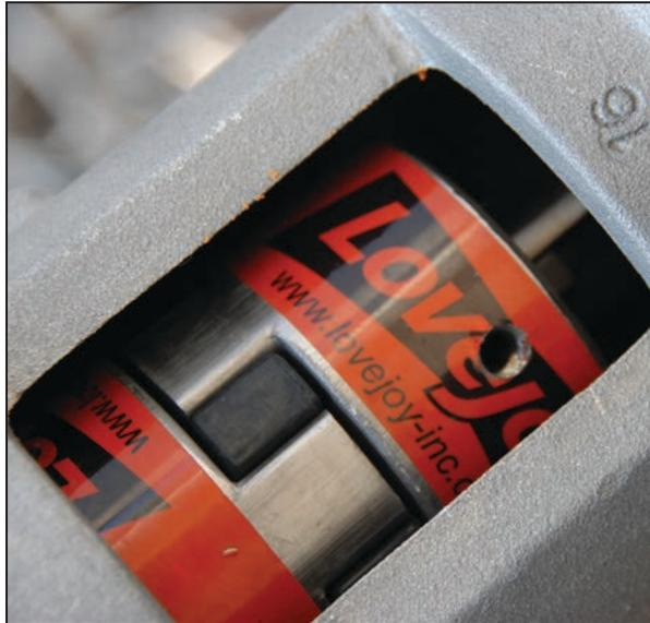
4. Loosen the setscrews in each coupling half and remove the old couplings.
