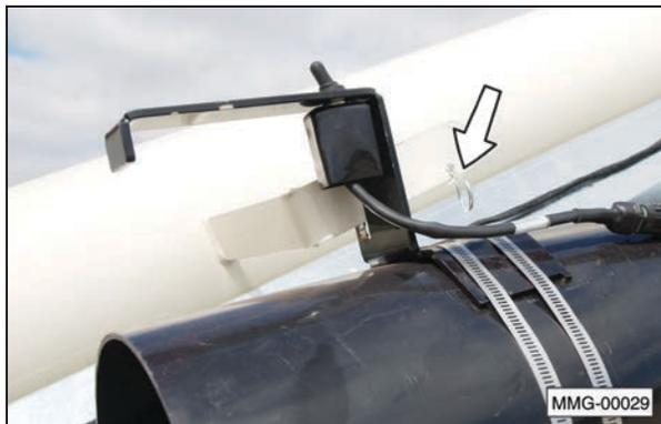
**NOTE:** When placing the conveyor tube in the storage position, make sure the pivot wheels are firmly seated against the platform. If too much downward pressure is applied to the conveyor tube, the pivot wheels will raise off the platform, as shown.
