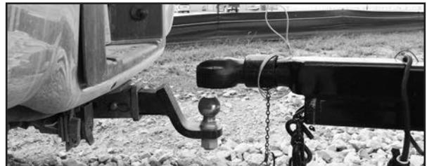
3. If equipped with an adjustable hitch, adjust the receiver height to make the trailer level with the tow vehicle. Tighten the bolts to standard torque for this size bolt.
