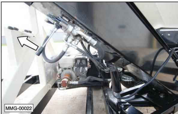
10. Set the conveyor belt speed control lever to the desired setting; 0 (zero) being no movement and 10 being full speed.
