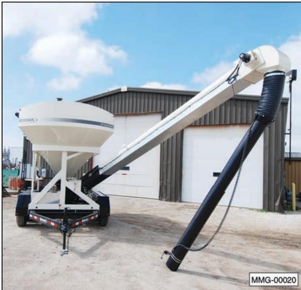
9. Raise or lower the conveyor tube to the desired height.
