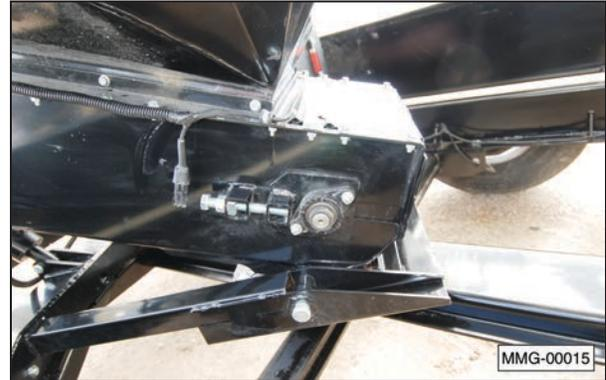
1. Loosen the locknut on each side of the belt tension mechanism.
