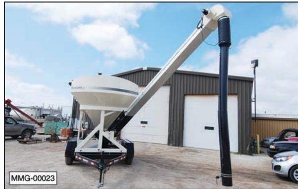
7. Using the conveyor tube raise/lower lever, slightly raise the conveyor out of the storage cradle.
