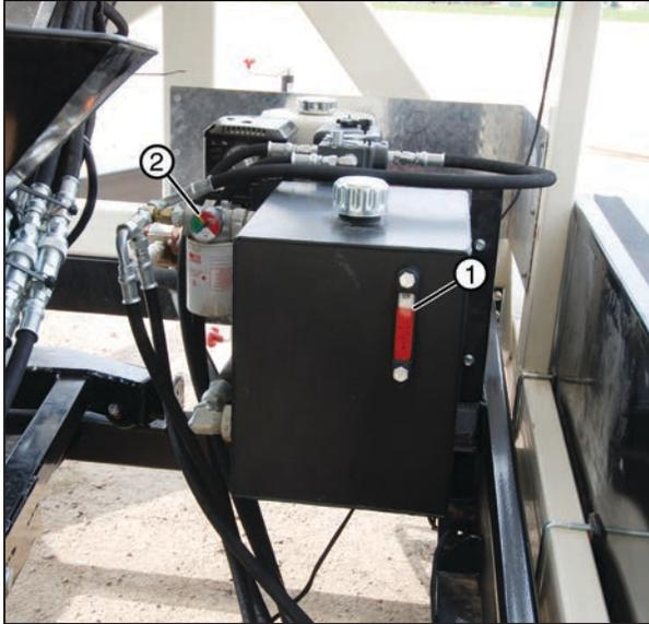
An oil and filter change is recommended annually or every 400 hours of operation using an AW HVI Hydraulic ISO 32 oil.
