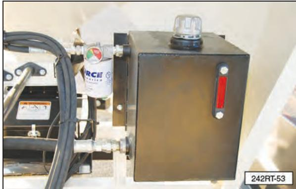
An oil and filter change is recommended annually or every 400 hours of operation using an AW HVI Hydraulic ISO 32 oil.
