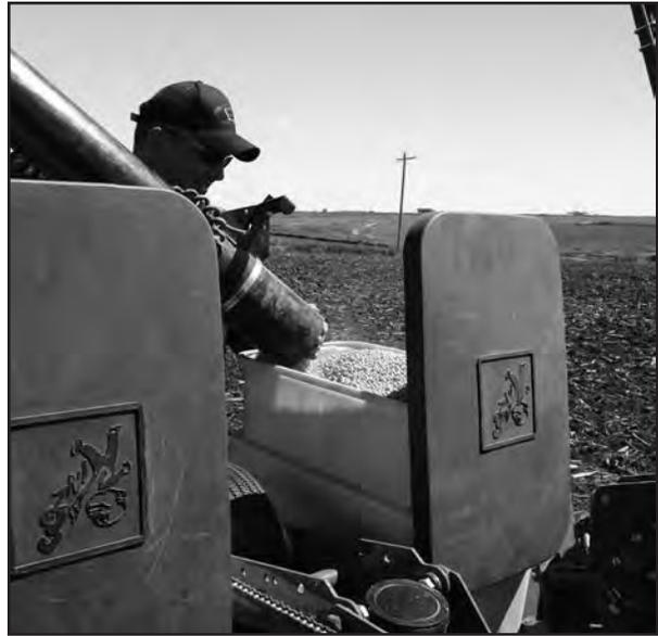
11. When finished loading the planter, return the conveyor to the transport position and install the lock pin and retaining clip.
