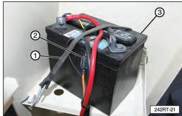
A 12 Volt battery (3) supplies the electrical power to start the gasoline engine and also to operate the solenoid valve that controls flow to the conveyor hydraulic motor. When the engine is operating, a trickle charge is sent to the battery to keep it fully charged. The rubber strap (1) is used to hold the battery in place. The fuse holder (2) contains a fuse for the power supply to the conveyor solenoid valve circuit.
