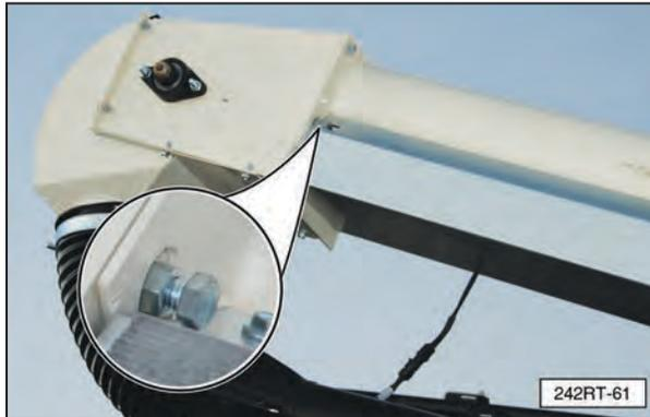
1. Loosen the locking nuts on the two adjusting bolts.
