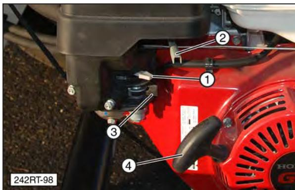
Each engine is equipped with a valve between the fuel tank and the carburetor. Slide the fuel shut-off valve (3) toward the engine to turn ON and away for OFF. Turn the fuel OFF when not in use or before transporting.
