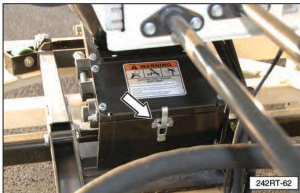
3. Position the lower roller adjusting bolts to their loosest position.
