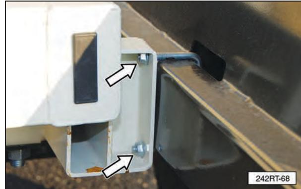
Check torque on axle mounting bolts. Tighten bolts to 290 ft-lbs..
