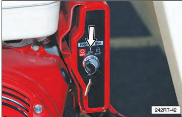
This key switch controls the power to the engine electrical system. Turn the key clockwise to the "START" position to crank the engine. When the engine starts, release the key and it will automatically return to the "ON" position. The key must be in the "ON" position for the engine to run. Turn the key counterclockwise to the "OFF" position to stop the engine.
