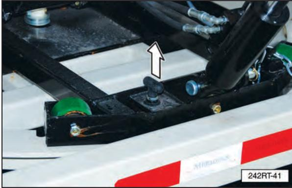
8. Start the conveyor by actuating the switch located at the end of the spout.
