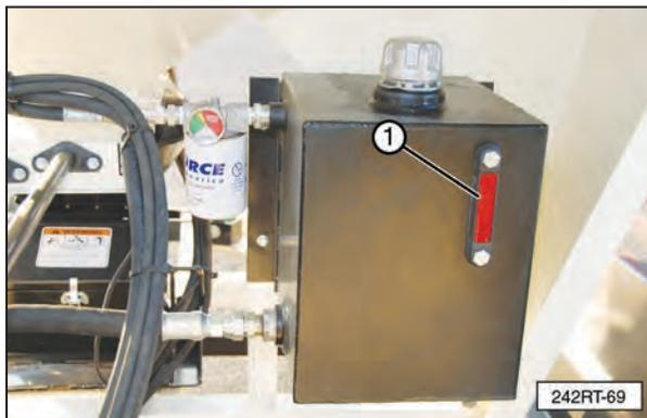
4. Check filter life indicator (2). Change the filter if the indicator needle is in the yellow or red area.
