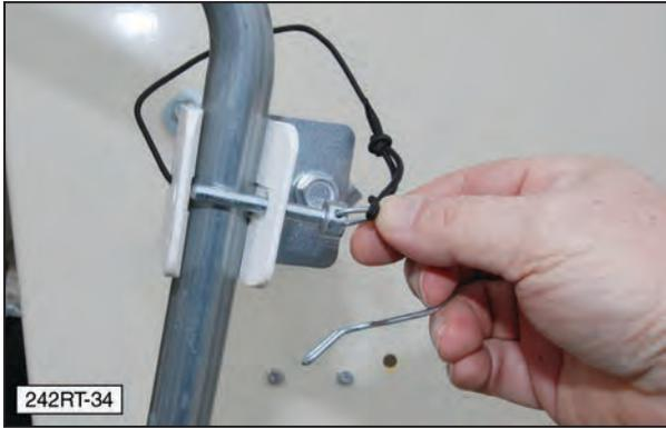
2. Extend the crank handle assembly to a comfortable operating position.
