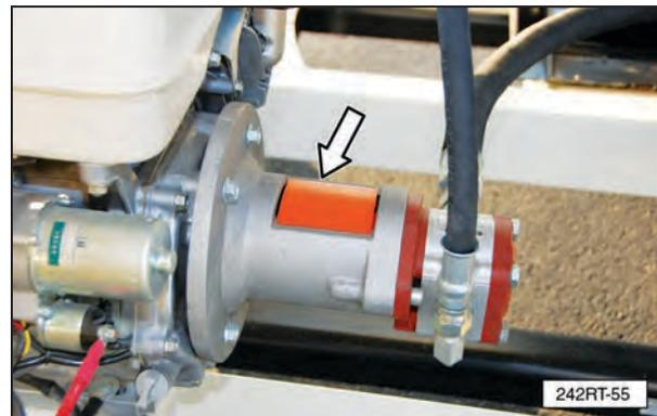
2. Remove the two pump mounting bolts.
