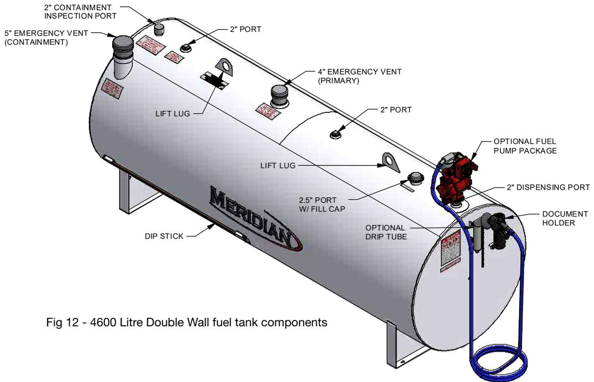
Fig 12 - 4600 Litre Double Wall fuel tank components
