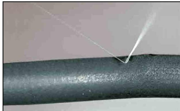
Fig 15 - Leak in transfer hose
