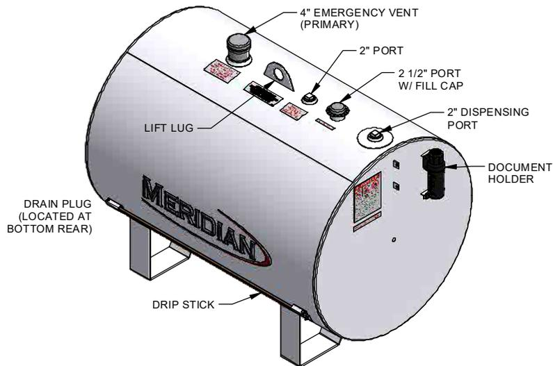
Fig 10 - 2300 Litre Single Wall Utility Tank components
