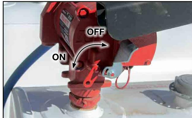
Fig 20 - Pump operation
