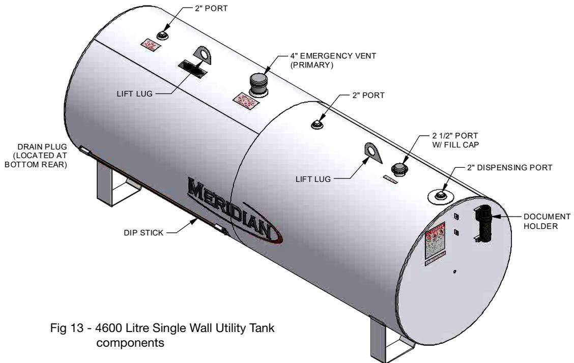
Fig 13 - 4600 Litre Single Wall Utility Tank components
