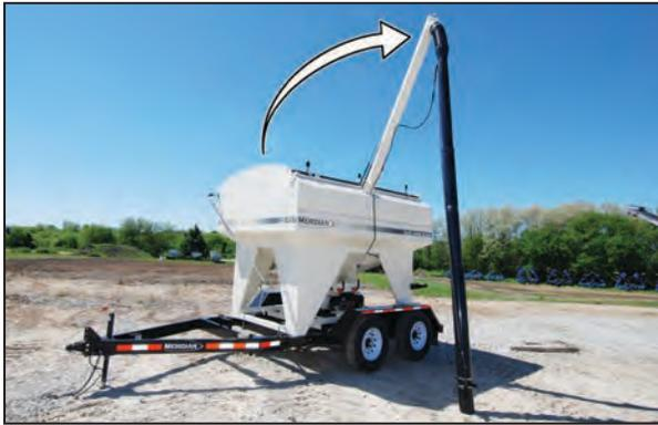
8. Lock the auger tube to the seed tender using the over-center clamp.
