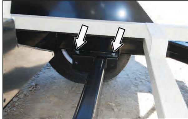
The front hitch section of the seed tender is bolted to the trailer frame. This design allows the same trailer to use either a standard bumper hitch assembly or a gooseneck trailer hitch if this option is available.
