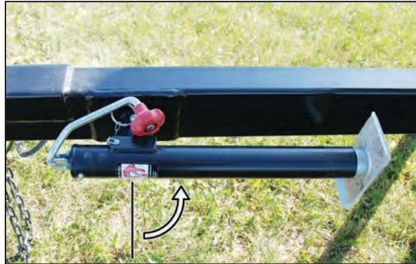
8. Close the receiver locking collar using the lever. Install the retainer clip to prevent unwanted opening of the receiver.
