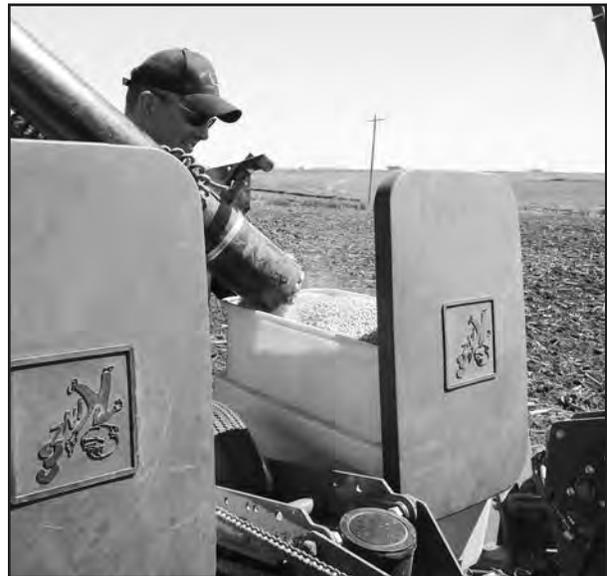
14. When the transfer of seed is complete, press the auger speed control switch to reduce the engine RPM and stop the auger.
