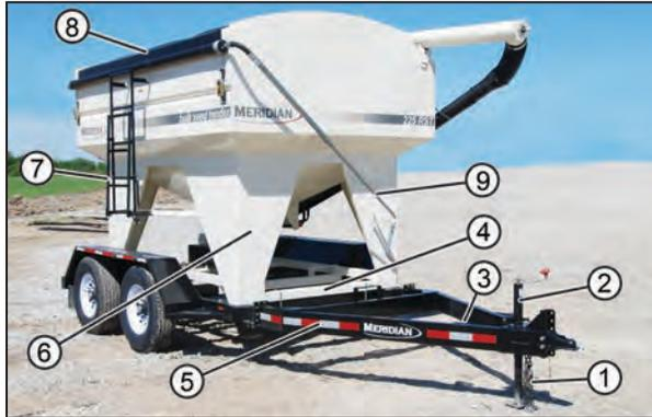
(1) Trailer Safety Chains. (2) Jack Stand. (3) Break-Away Trailer Brake System. (4) Seed Tender Frame. (5) Trailer. (6) Document Storage Tube (inside of frame). (7) Ladder. (8) Seed Bin Cover. (9) Cover Open/Close Bar.
