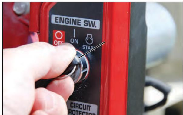
11. If necessary, decrease the engine speed below 1400 RPM using the remote throttle control switch. A centrifugal clutch on the engine will engage and rotate the auger when the engine speed exceeds 1400 RPM. Increasing the engine speed will increase the unloading rate.
