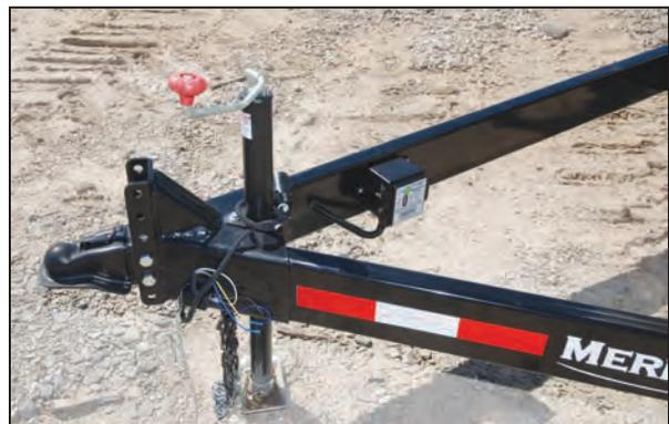
3. Adjust the receiver height to make the trailer level with the tow vehicle. Tighten the bolts to 70 ft-lb (95 N·m) torque.
