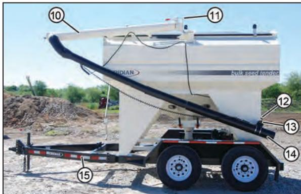
(10) Auger Tube. (11) Auger Tube Clamp. (12) Delivery Spout Holder. (13) Auger/Engine Throttle Switch. (14) Delivery Spout. (15) Bolt-On Bumper Hitch Tongue Assembly.
