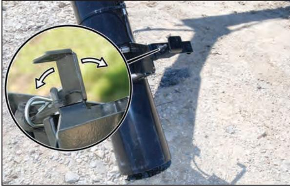
12. Open the seed compartment slide gate by pushing the handle inward. Close the slide gate by pulling the handle outward.
