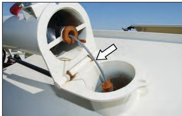
7. Raise the auger tube by pushing it upward, using the delivery spout. A small gas-filled shock will assist in raising the auger tube.
