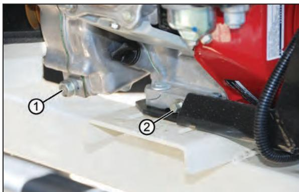
5. Reinstall the drain plug and tighten.
