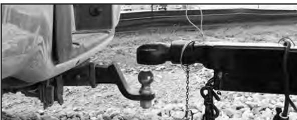
6. Lower the hitch onto the ball.
