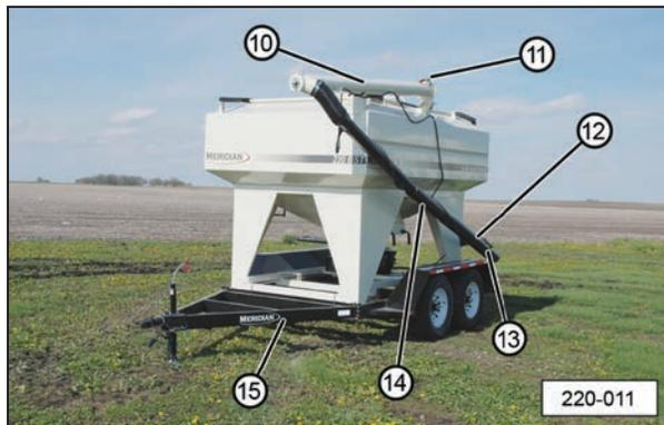
(10) Auger Tube. (11) Auger Tube Clamp. (12) Delivery Spout Holder. (13) Auger/Engine Throttle Switch. (14) Delivery Spout. (15) Bolt-On Trailer Tongue Assembly.
