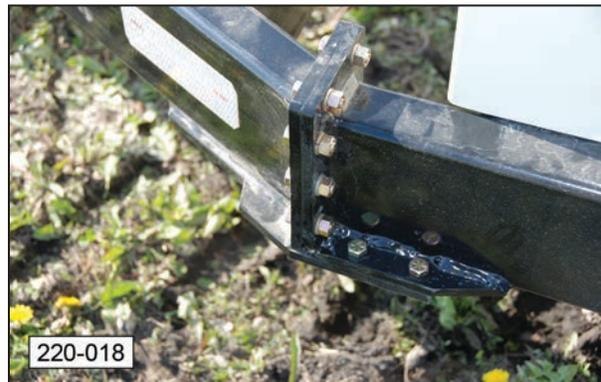
Check the torque on the frame hold-down bolts at least once per year. Tighten the bolts to 40 ft-lbs.
