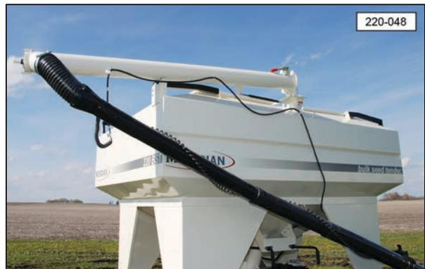
6. Make sure the auger cable is threaded into the hole in the end of the auger. Damage to the auger can occur if the cable is not properly inserted.
