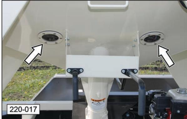
4. When the compartment is filled, close the cover(s) and lock it in place with the rubber latch.
