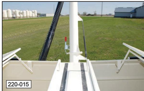
**Note:** Before filling the seed compartment, make sure the seed delivery chutes are open/unblocked.
