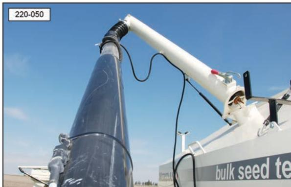
9. Place the delivery spout onto the storage bracket and secure it with the rubber strap.
