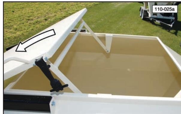
5. When the bin is filled, close the cover and lock it in place with the rubber latch.
