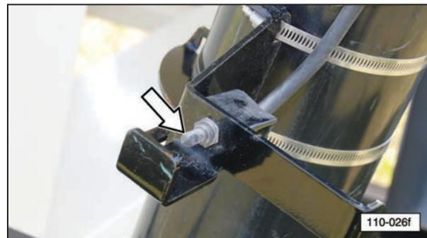
13. Open the seed slide gate by pushing the handle inward. Close the seed slide gate by pulling the handle outward.
