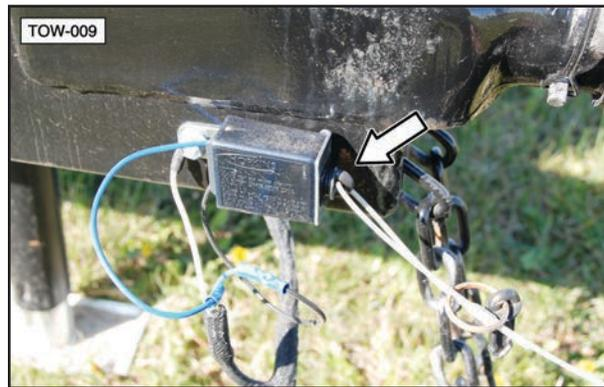
11. Route all the cables in a manner that will prevent snagging. Be sure to provide slack for turning.
