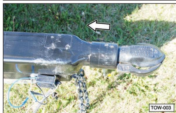
4. Slowly back the tow vehicle until the hitch and ball are aligned.
