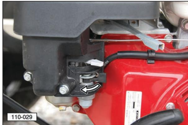
19. Before towing the unit on the road, return the auger tube and delivery spout to its stored position. Latch the rubber tie-down strap over the delivery spout.
