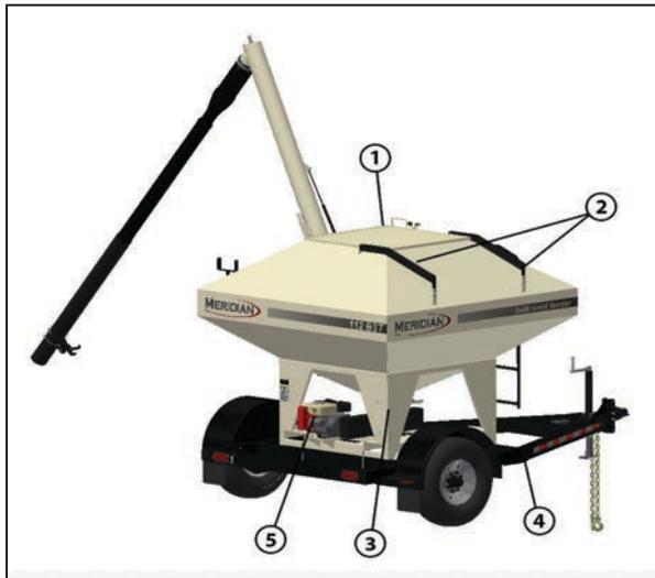
(1) Seed Bin Cover. (2) Seed Bin Cover Rails. (3) Seed Tender Frame. (4) Trailer. (5) Gasoline Engine.
