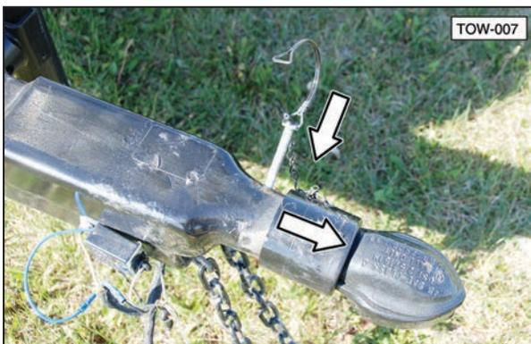
8. Attach the safety chain securely to the tow vehicle to prevent unexpected separation. Cross the chains when attaching.
