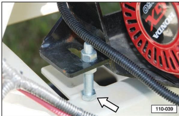
3. Loosen the engine base adjusting bolt jam nut and move the engine base to set the desired belt tension.
