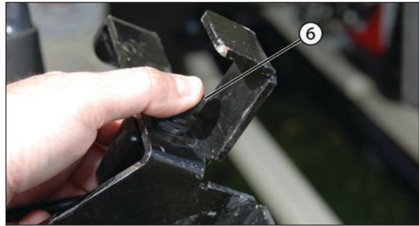
3. Ensure all personnel are clear of unit. Start the engine and test the actuator by pressing actuator switch (6) to ensure the engine speed increases and decreases as designed.
