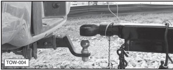
5. Lower the hitch onto the ball.
