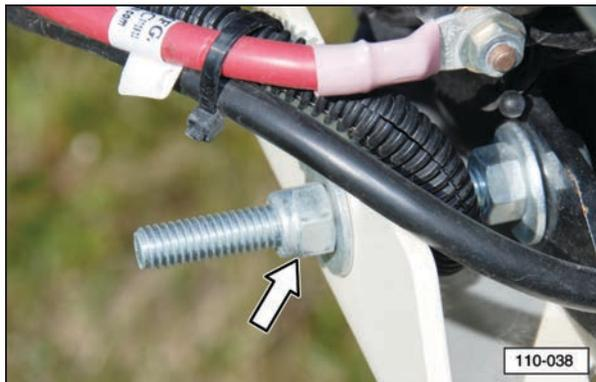
4. Tighten the jam nut.
