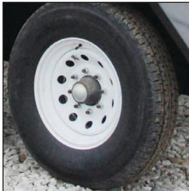
1. Initially check the wheel bolt torque at 10, 25, and 50 miles and after each wheel removal. Refer to the Wheel Bolt Torque Requirements section in this manual for tightening instructions.
