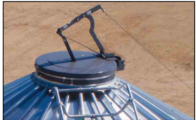
Fig 9 - Loading hatch covered by the lid
