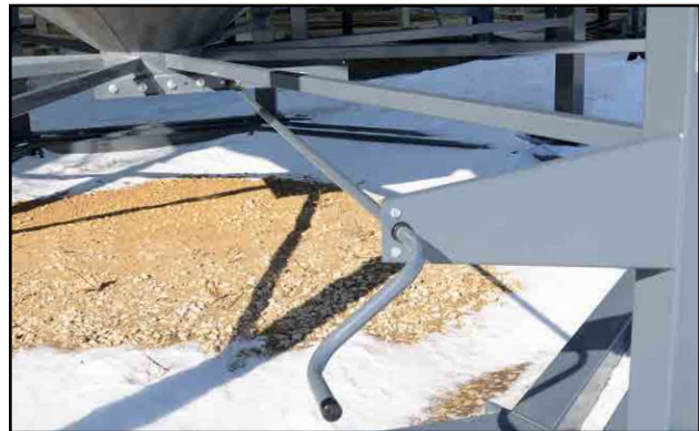
Fig 6 - Unloading chute with slide gate and crank
