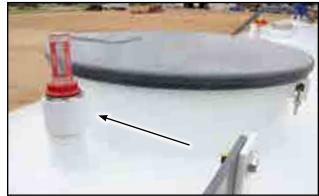
Fig 9 - Containment Inspection Port w/ Leak Detection Gauge
