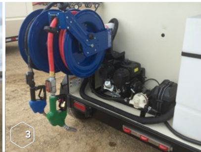
6.5hp Gas Engine, 40GPM Pump c/w 25'x3/4" Hose, Meter, Auto Nozzle, Auto Reels & 208L DEF System
